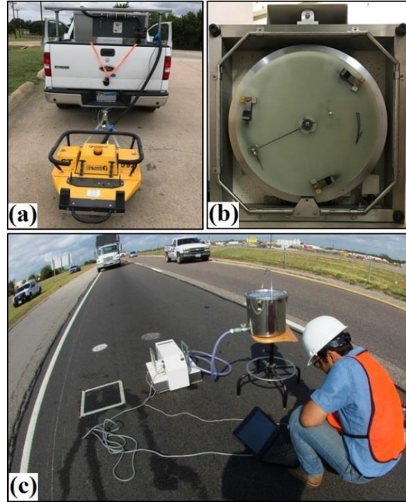
Figure 4.1 a) The Grip-Tester attached to a vehicle, b) bottom view of the DFT, and c) the DFT connected to a water tank and DCC measuring the friction at the lane center path
