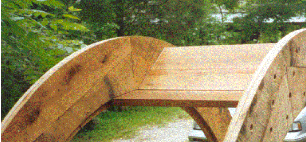
Figure 50. A bucket and sole plate, showing why the edges of the buckets are beveled.
