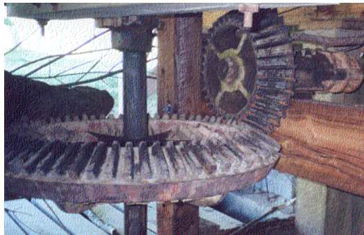
Figure 114. Large bevel gears transmitting power from the turbine to mill machinery, located at Ketner's Mill in Marion County, Tennessee. The lower gear has wooden cogs.
