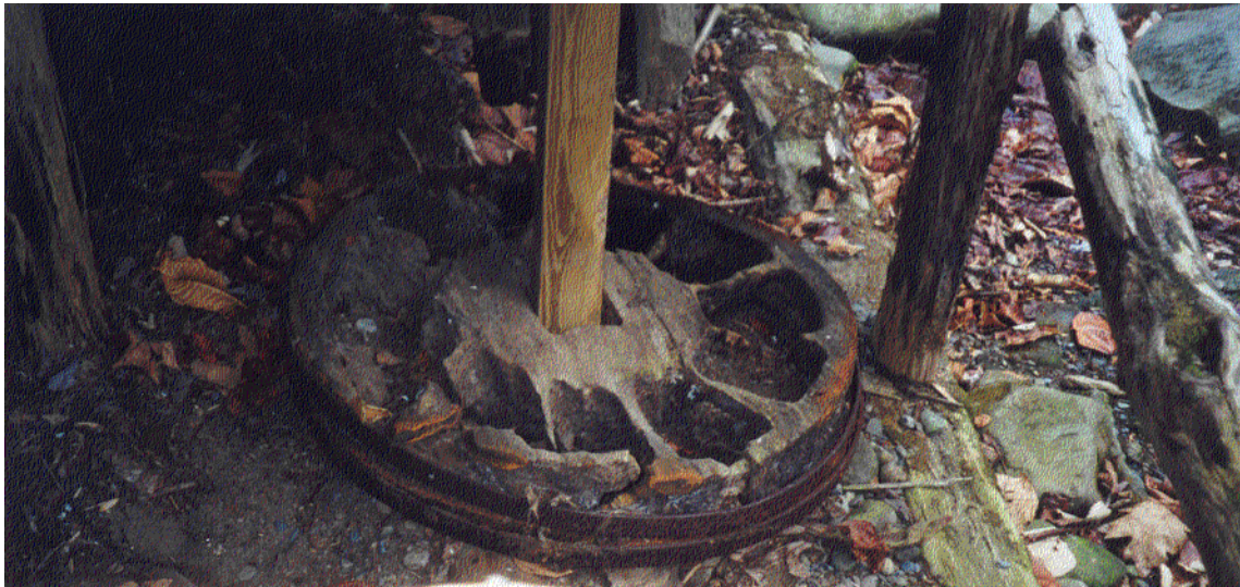
Figure 38. Tub wheel at Ogle Tub Mill in Great Smoky Mountain National Park.
