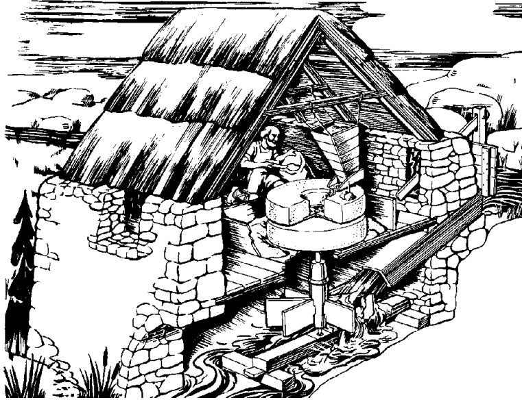
Figure 3. Primitive turbine with millstones directly connected.
