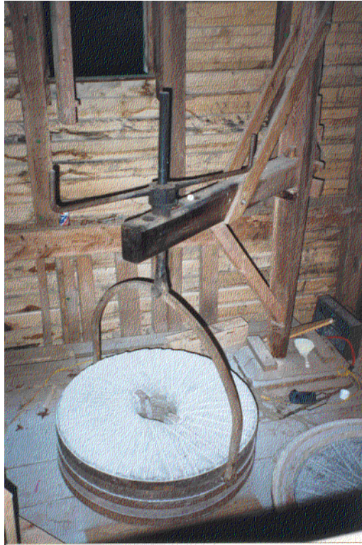
Figure 93. The crane, lifting screw, crank, and bails secured to the runner stone. The runner has been lifted off the bedstone, turned over, and swung clear for dressing.
