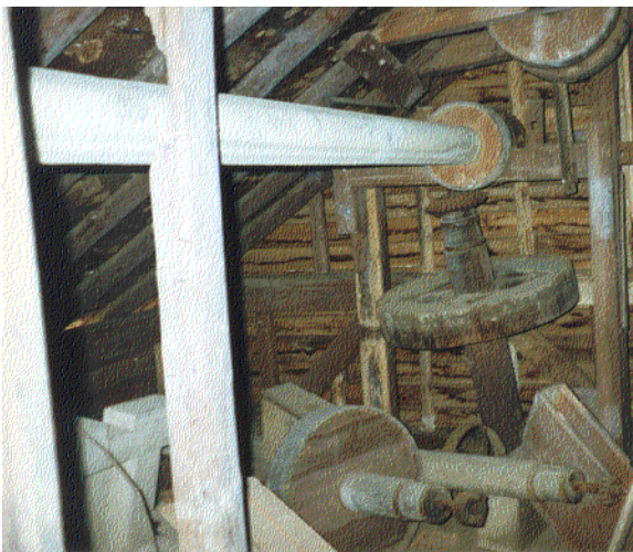
Figure 111. Wooden shafts and pulleys in a pre-Civil War mill (Selma, AL)
