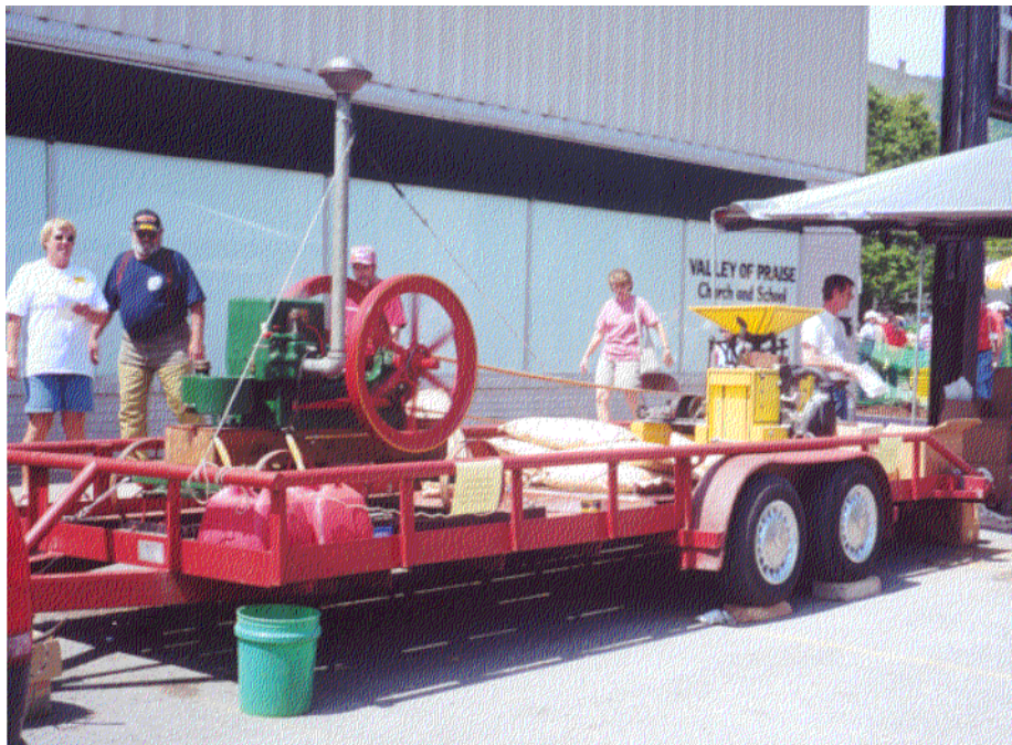
Figure 139. A very cantankerous 1916 Witte 6 horsepower, one-cylinder gasoline engine, restored by the author and used to power an early Williams stone buhr mill.
