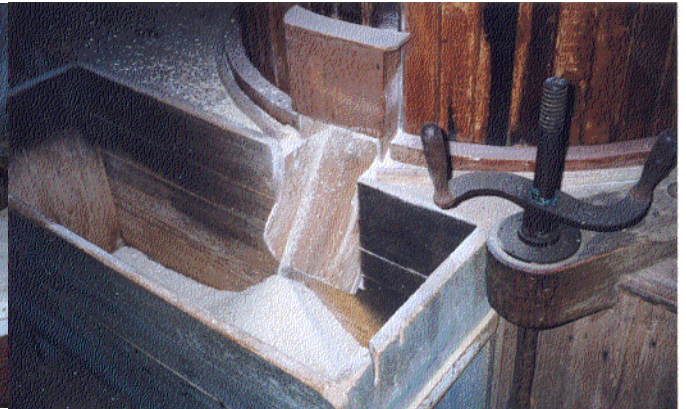
Figure 102. Meal emerges from spout. Note tentering screw and crank.
