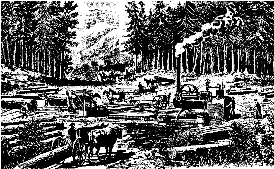
Figure 89. Portable Case sawmill and skid-mounted steam engine of 1882.
