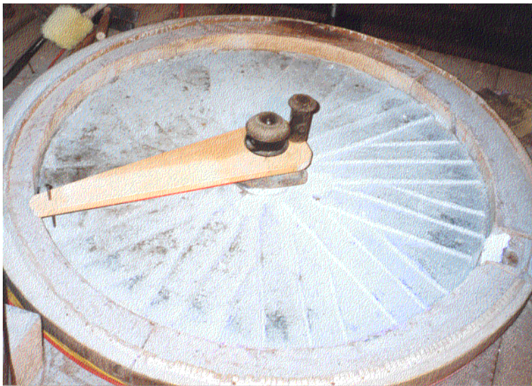
Figure 42. Trammimg the millstone shaft with a wooden device called a trammel.
