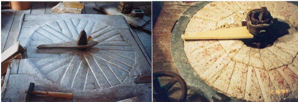
Figure 4. Monolithic native granite millstone on left; segmented French buhrstone on right. Both stones have trammels in place for checking shaft perpendicularity to bedstone.
