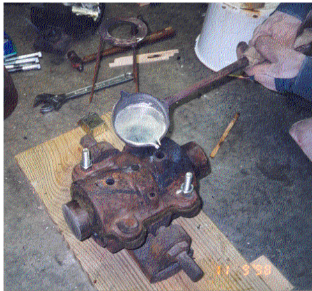
Figure 113. Pouring a babbitt bearing. The base has been poured, the cap dammed and positioned, and the molten metal is poured through one of the oil holes.
