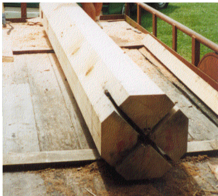
Figure 44. An 18-inch octagonal white oak water wheel axle showing gudgeon mortises.
