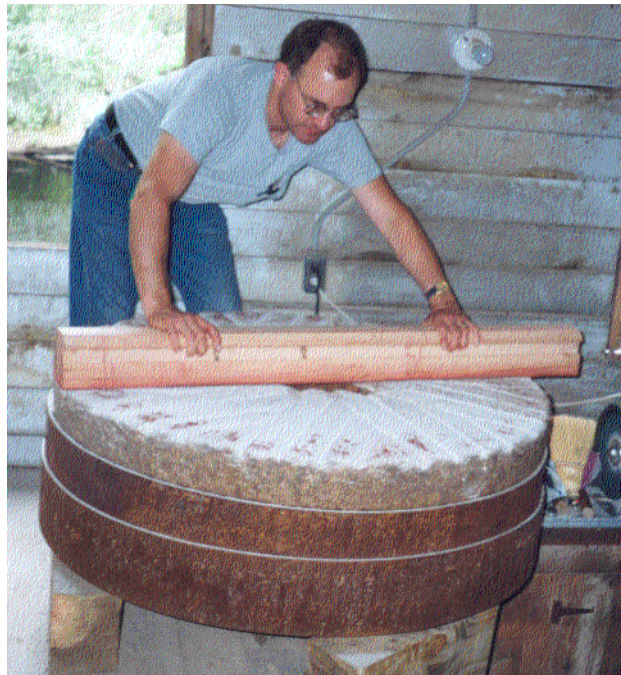
Figure 97. “Staffing” the runner stone with the dye, or paint, staff. Notice the presence of dye on the outer six inches or so of the face of the stone, which is desirable.
