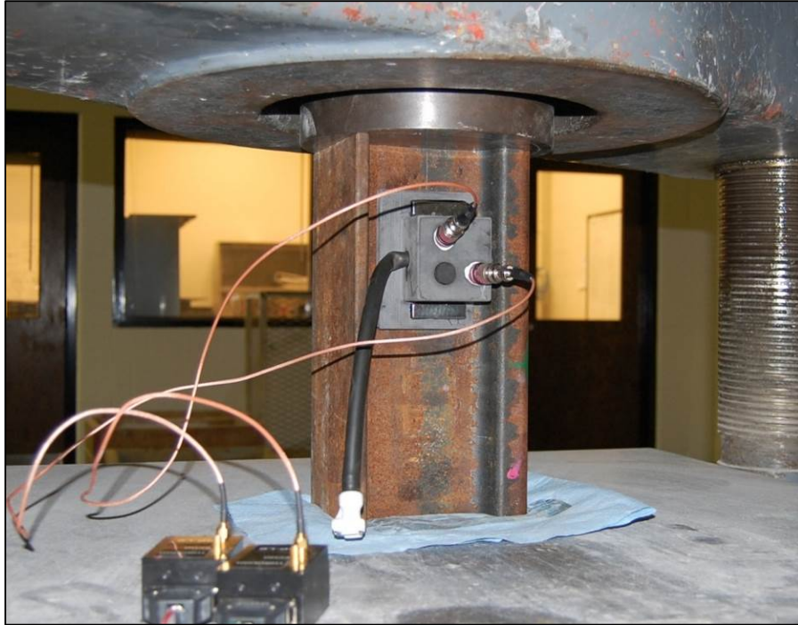
Figure 38. Loading Ram Compressing the Rail Section While Two Shear Transducers Are Used to Monitor the Backscatter Signals
