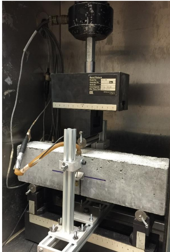
Figure 3.9 Testing equipment setup for fracture test
