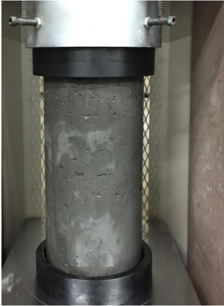
Figure 3.3 Compressive strength test
