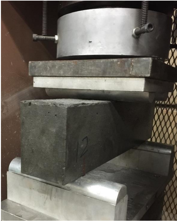
Figure 3.5 Flexural strength test (3 inch \times 4 inch \times 16 inch prism, span: 12 inch)
