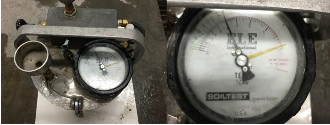
Figure 3.2 Air content test by pressure method
