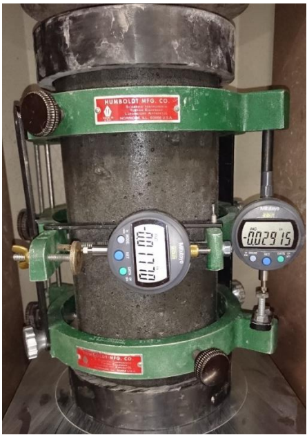
Figure 3.4 Modulus of elasticity test
