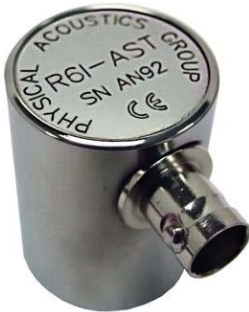
Figure 5: Photographs of some of the AE probes used in the experiments. The first two probes are wide band probes, with frequency response extending to 900 kHz and the third probe is a resonant probe (60 kHz) that provides better sensitivity.
