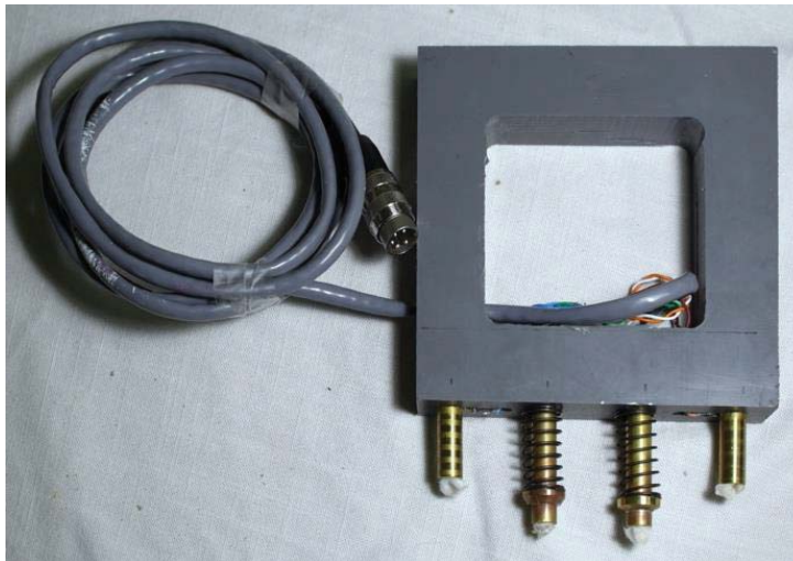
Figure 12: Photograph of the Wenner array probe fabricated in the laboratory for the measurement of resistivity in the concrete block
