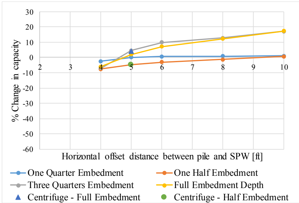
Figure 6.3 Variation of ultimate capacity in Scenario 3 with respect to horizontal offset distance (feet) and SPW embedment depth normalized by pile tip depth
