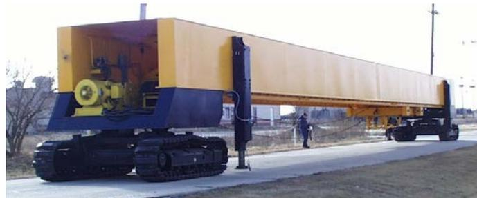
Accelerated Transportation Loading Assembly (ATLAS) at ICT
