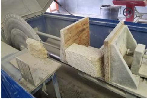
Saw-cutting cubes for strength testing
