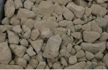
Aggregate subgrade/ QB blends with 30% oven-dried QB, by weight
