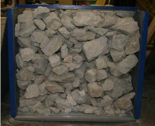
Aggregate subgrade compacted in two lifts
