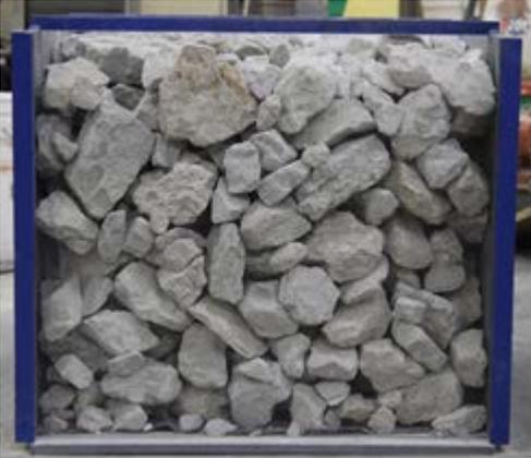
Aggregate subgrade compacted in one lift
