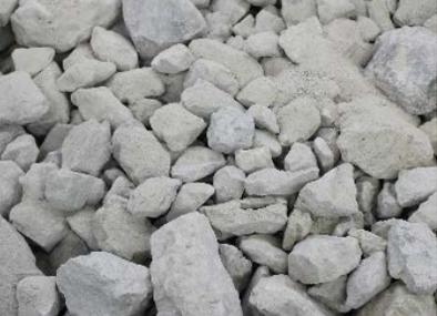
Aggregate subgrade/ QB blends with 20% oven-dried QB, by weight
