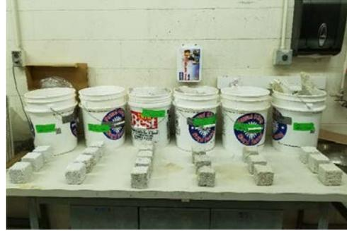
Saw-cut cubes from different sections
