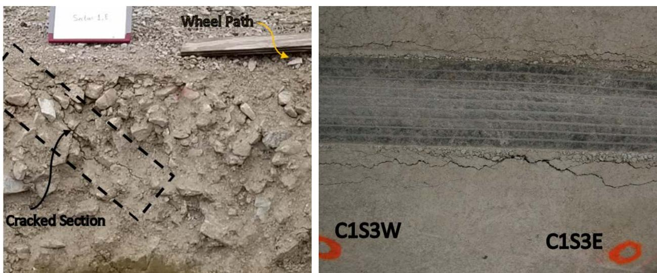
Cracking in C1S1E (PCR/QB1 – 2 Lifts)
