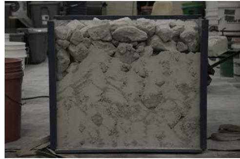
Aggregate subgrade/ QB blends with 30% oven-dried QB, by weight compacted in one lift
