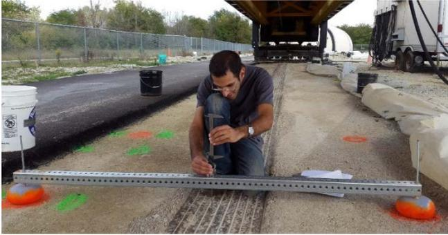
(a) Customized Rut Depth Measuring Device
