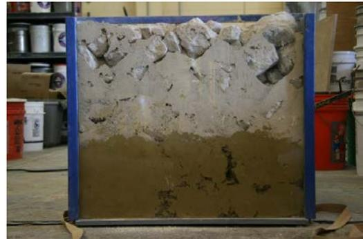
Aggregate subgrade/ QB blends with 25% wet QB (moisture content = 2.5%), compacted in two lifts
