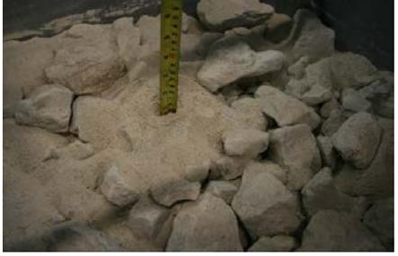
Aggregate subgrade/ QB blends with 40% oven-dried QB, by weight
