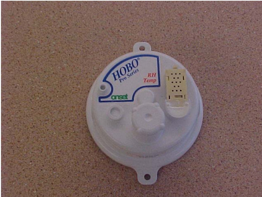
Figure 3.6 HOBO ® H8 Pro RH/Temperature Loggers
