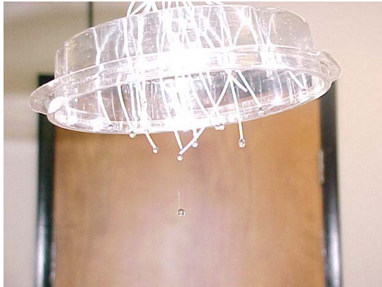
Figure 3.16 Photo of nozzle for distributing leaching media into column leaching test apparatus.
