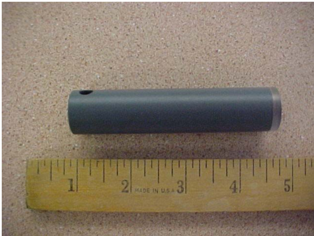
Figure 3.7 Vemco ® Minilog Temperature Probe
