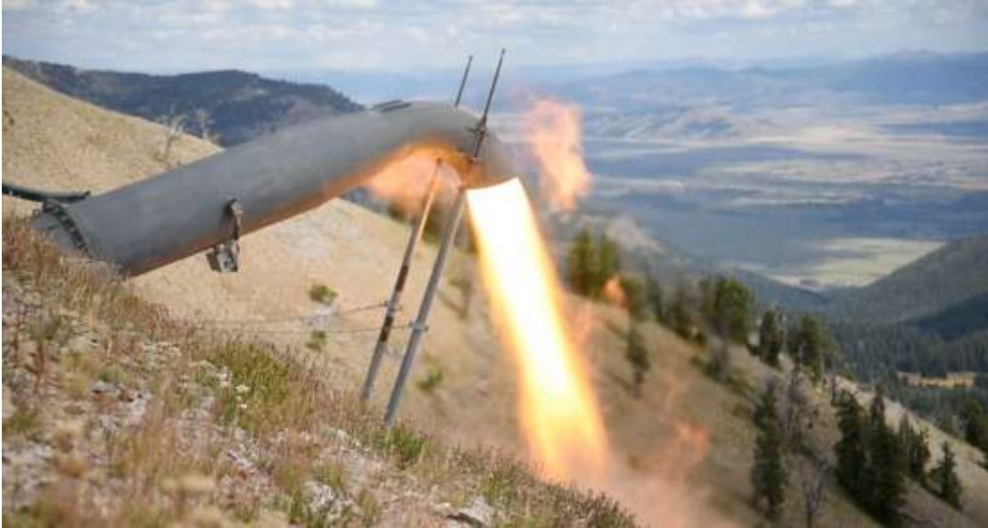
Figure 14. A summer test firing of a GAZEX® in the avalanche-starting zone above State Route 22, Teton Pass, Wyoming.
