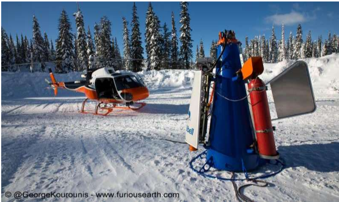
Figure 18. A modified gas exploder, the TAS Daisy Bell®, is portable and can be fired from its sling cable below a helicopter.
