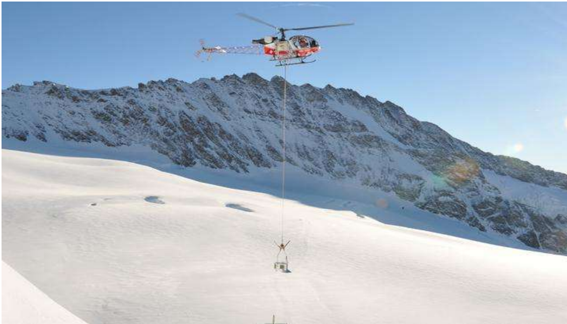
Figure 6. The Wyssen Avalanche Control explosive delivery technology is also portable and explosives can be dropped from it while it is hanging from a sling cable below the helicopter.
