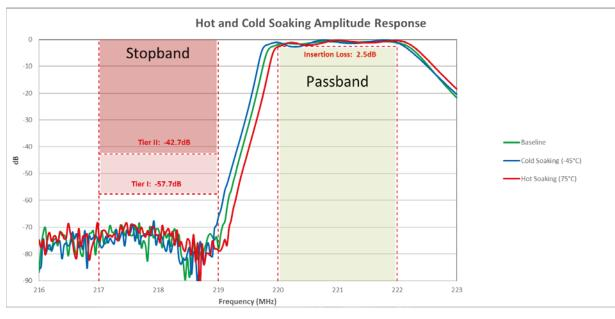
Figure 4. Vendor B ITC Amplitude Response for Temperature Extreme Tests
