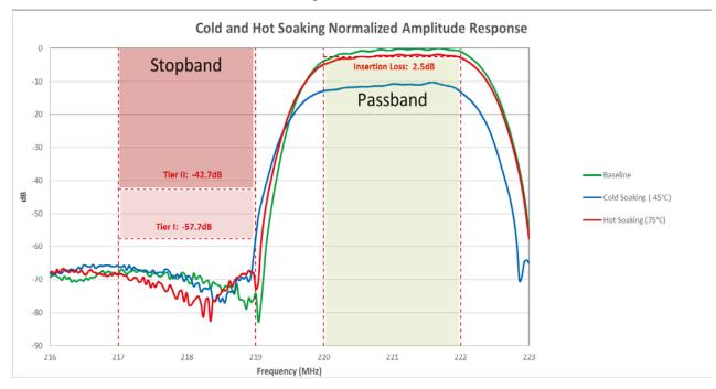
Figure 2. Vendor A ITC Amplitude Response for Temperature Extreme Tests
