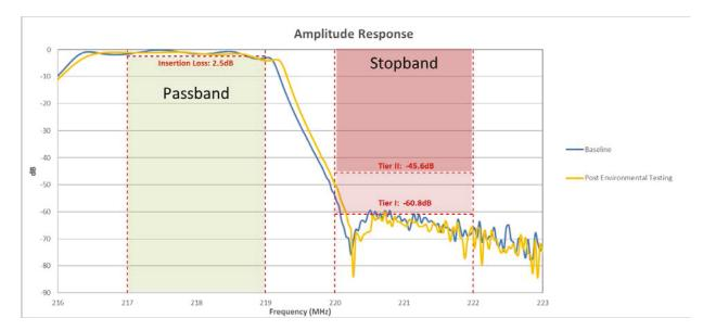
Figure 16. Vendor D Amplitude Response ACSES Filter Characterization
