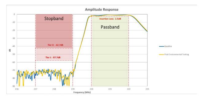
Figure 3. Vendor B Amplitude Response ITC Filter Characterization
