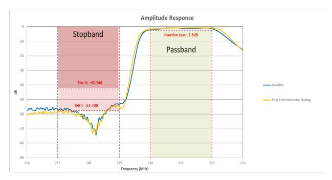
Figure 9. Vendor H Amplitude Response ITC Filter Characterization
