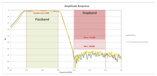
Figure 14. Vendor B Amplitude Response ACSES Filter Characterization
