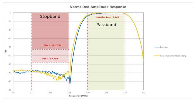
Figure 1. Vendor A Amplitude Response ITC Filter Characterization
