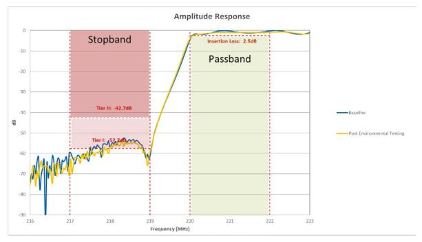
Figure 5. Vendor D Amplitude Response ITC Filter Characterization
