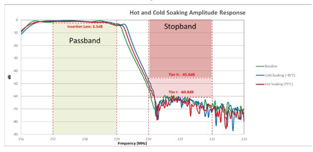
Figure 17. Vendor D ACSES Amplitude Response for Temperature Extreme Tests
