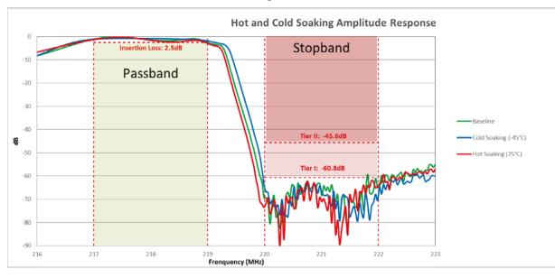
Figure 19. Vendor F ACSES Amplitude Response for Temperature Extreme Tests
