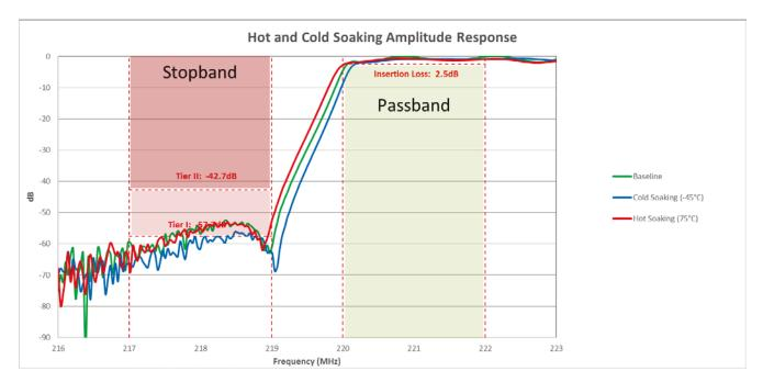
Figure 6. Vendor D ITC Amplitude Response for Temperature Extreme Tests
