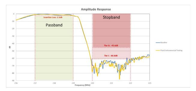
Figure 18. Vendor F Amplitude Response ACSES Filter Characterization
