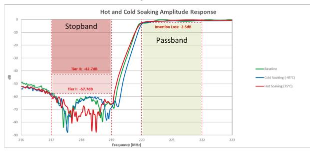
Figure 8. Vendor F ITC Amplitude Response for Temperature Extreme Tests
