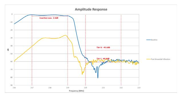
Figure 20. Vendor H Amplitude Response ACSES Filter Characterization
