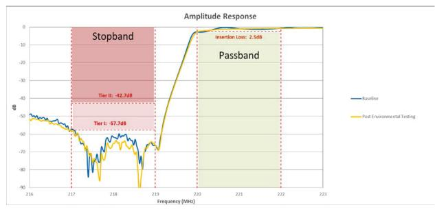
Figure 7. Vendor F Amplitude Response ITC Filter Characterization
