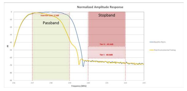
Figure 11. Vendor A Amplitude Response ACSES Filter Characterization
