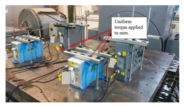
Figure 22. Side Mounting Used for Testing
