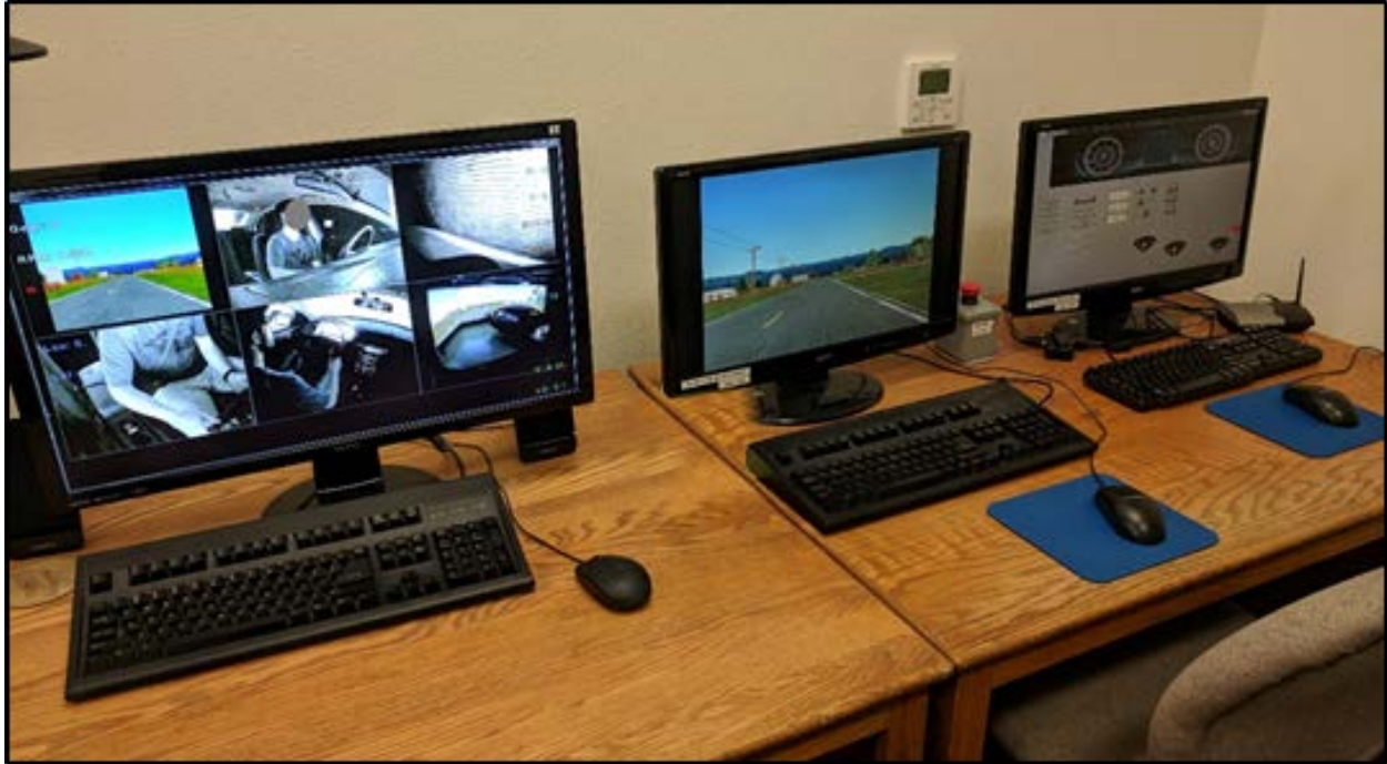
Figure 3.3: Operator workstation for the full-scale driving simulator. Monitors are shown displaying SimObserver (left), and the simulated environment (center) or vehicle dashboard (right) as seen in the vehicle.
