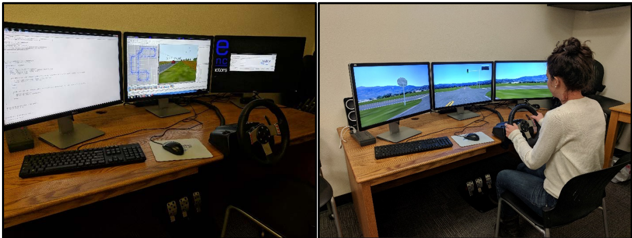
Figure 3.1: Operator workstation for the driving simulator. Left: Designing an experiment in the Internet Scene Assembler with Java script. Right: A researcher evaluating a newly designed environment.
