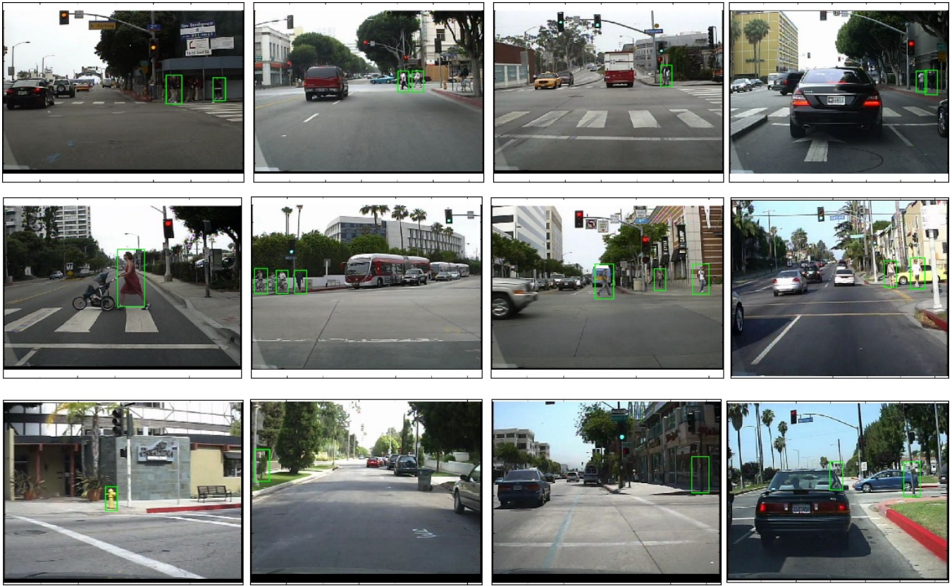
Fig. 6. Qualitative detection results on the Caltech testset. The first and second row shows correct pedestrian detections in various scenarios. The third row shows typical false positives.
