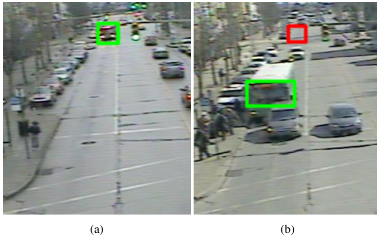
Figure 1: Qualitative results. (a) A tiny bus detected with score 1.000. (b) An occluded bus detected with score 1.000 shown in green and a false positive with score 0.926 shown in red. Figure 7 suggests that this is a very low false positive score.
