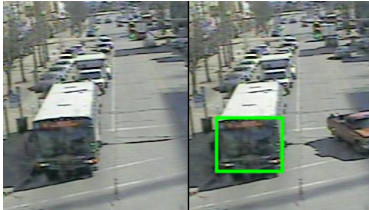
Figure 6: Effect of sampling. The same bus detected in one case but missed in another.
