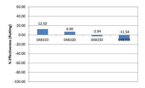
Figure 46. Treatment Effectiveness Based on Rutting for 04B300 Sections, 1991
