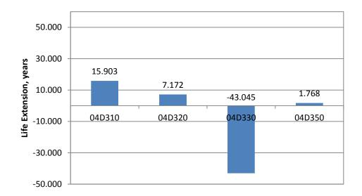
Figure 38. Life Extension Based on Environmental Damage Index for 04D300 Sections
