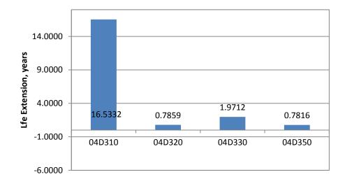
Figure 39. Life Extension Based on Rutting for 04D300 Sections
