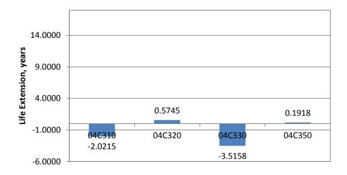
Figure 36. Life Extension Based on Rutting for 04C300 Sections
