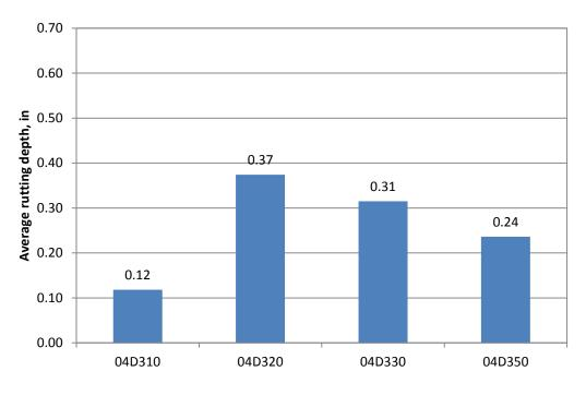
Figure 27. Average Rutting Depth for 04D300 Sections
