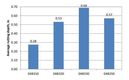
Figure 19. Average Rutting Depth for 04B300 Sections
