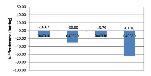
Figure 50. Treatment Effectiveness Based on EDI for 04C300 Sections
