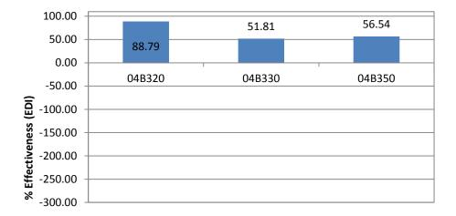
Figure 48. Treatment Effectiveness Based on EDI for 04B300 Sections, 1994
