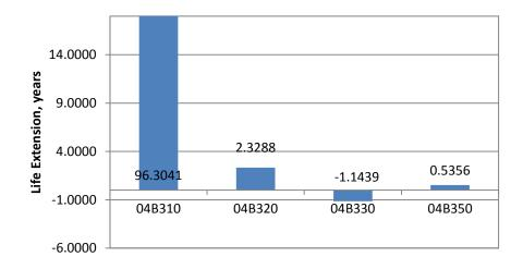
Figure 33. Life Extension Based on Rutting for 04B300 Sections
