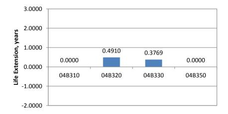
Figure 31. Life Extension Based on Structural Damage Index for 04B300 Sections
