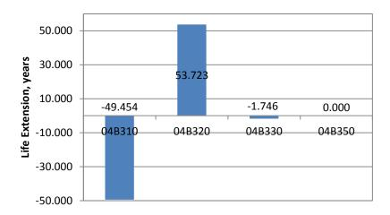
Figure 32. Life Extension Based on Environmental Damage Index for 04B300 Sections
