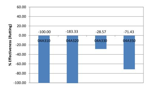
Figure 43. Treatment Effectiveness Based on Rutting for 04A300 Sections
