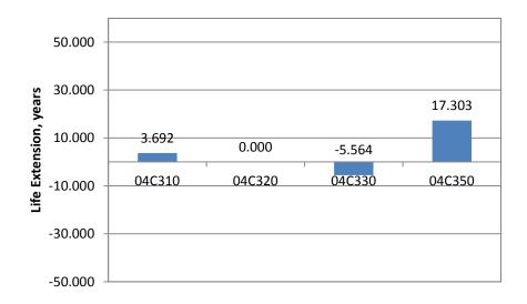
Figure 35. Life Extension Based on Environmental Damage Index for 04C300 Sections
