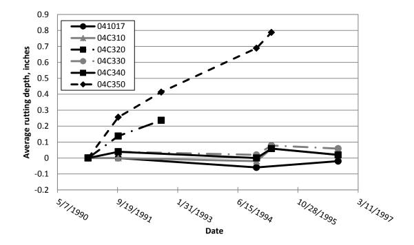
Figure 10. Rutting Trends for 04C300 Sections
