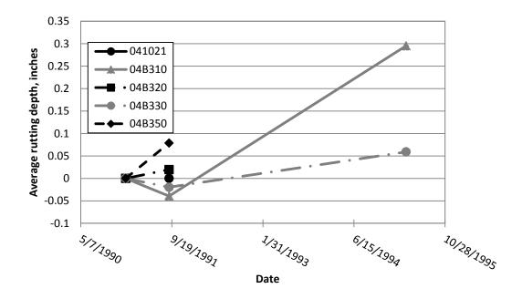
Figure 7. Rutting Trends for 04B300 Sections
