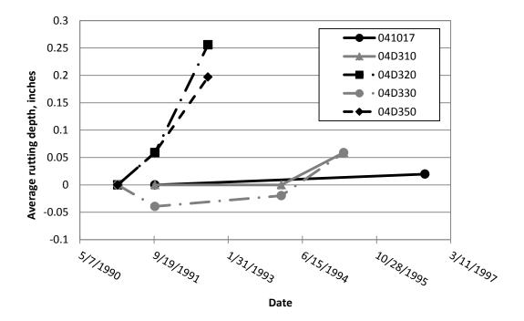
Figure 13. Rutting Trends for 04D300 Sections
