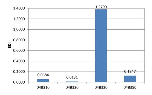
Figure 18. Environmental Damage Index for 04B300 Sections
