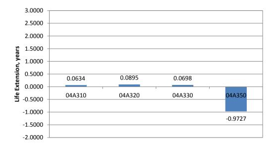
Figure 28. Life Extension Based on Structural Damage Index for 04A300 Sections
