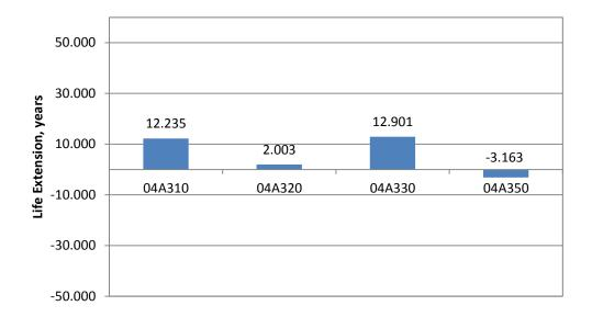
Figure 29. Life Extension Based on Environmental Damage Index for 04A300 Sections
