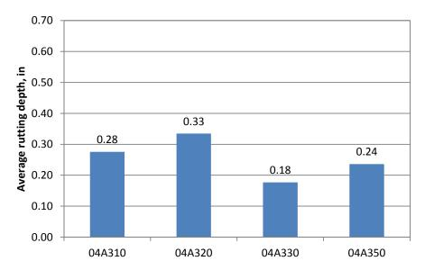
Figure 16. Average Rutting Depth for 04A300 Sections
