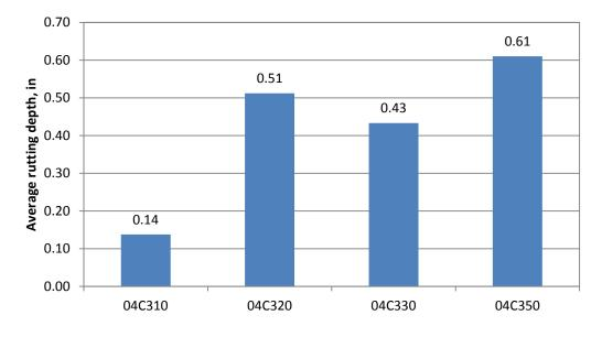
Figure 24. Average Rutting Depth for 04C300 Sections
