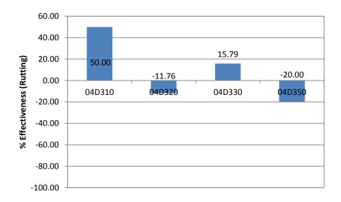
Figure 54. Treatment Effectiveness Based on Rutting for 04D300 Sections
