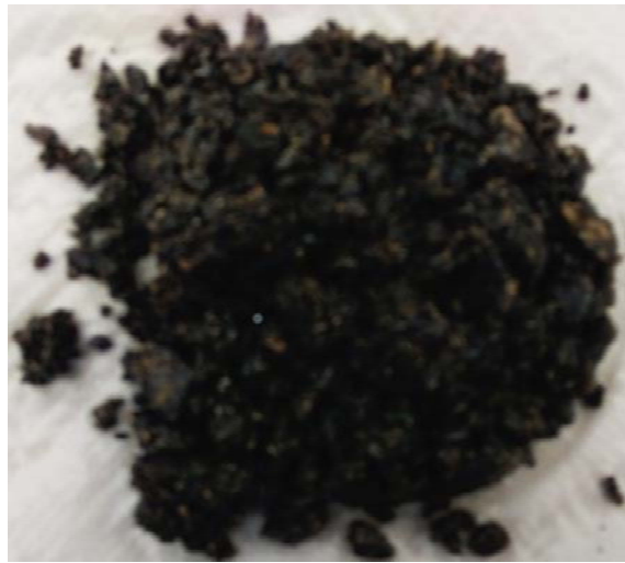
Figure 5-30 Stripped Surface Type B Mixtures from Various Aggregate Sources (A, C and E) after Boiling Test Procedures: (a)-(c)
