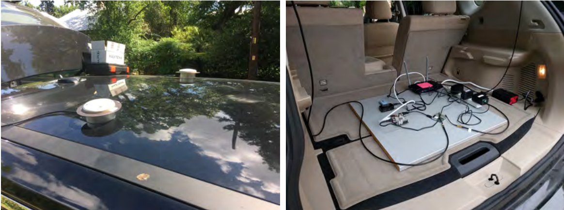
(a) Two-antenna set up on roof of the demonstration vehicle for two-antenna RTK and spoofing detection. (b) Electronics hub in demonstration vehicle trunk. Includes CDGNSS receiver, smartphone processor, and WiFi router.
