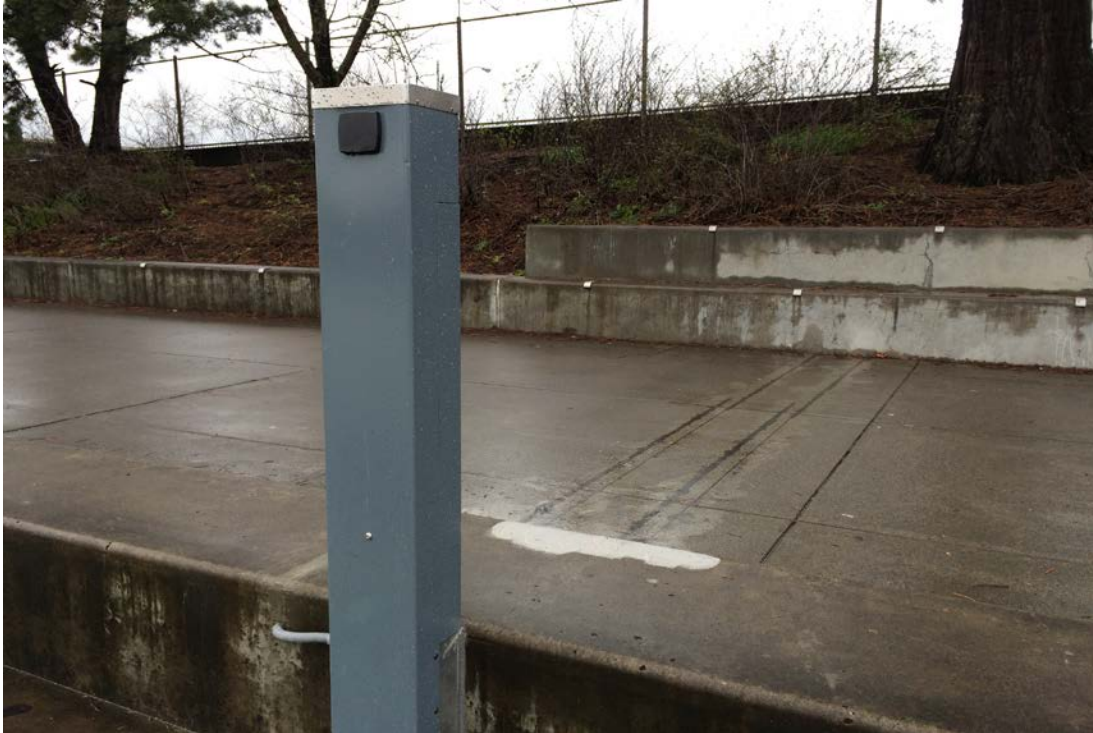
Figure 14 Piezoelectric and passive infrared combo on the Eastbank Esplanade.
