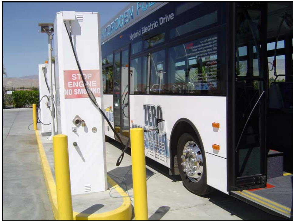
Figure 3. Fuel Cell Bus at Hydrogen Dispenser
