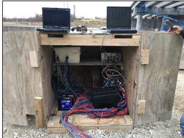
Figure 13. View of multiplexers and datalogger in use collecting data.
