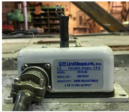
Appendix Figure H.5. UniMeasure ® string potentiometer.
