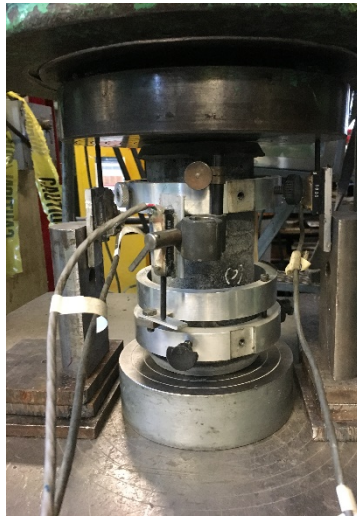
Elastic Modulus Cylinder
