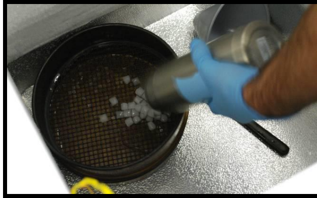
Figure 5.5 Separating the ice from the liquid
