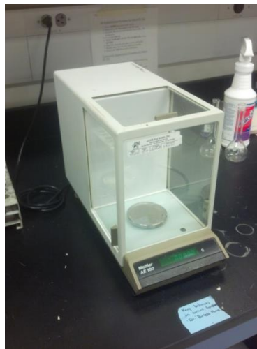
Figure 5.2 Digital mass balance in confining glass box
