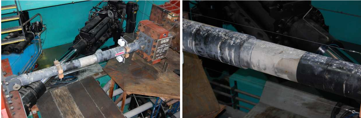
Figure 7. Overview of SN#004 as mounted for testing and leaking at the threaded connection.
