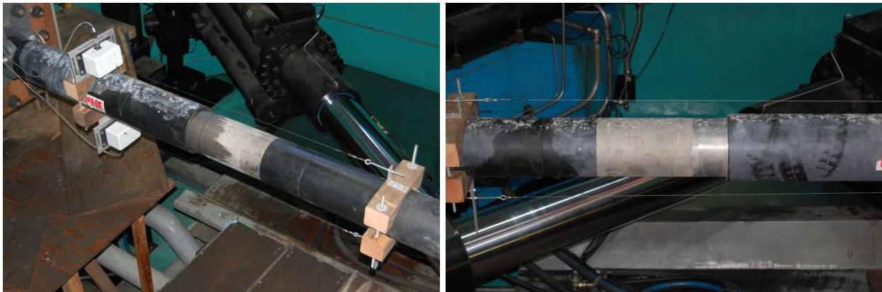
Figure 8 a) SN#006 leaking at the sleeve cover, b) SN#001 leaking at the threaded connection
