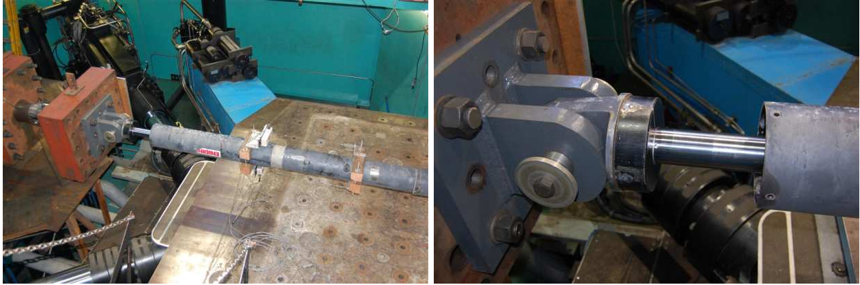
Figure 13. (a) Overview of stripped sleeve, and (b) close up of sheared bolts on SN#003 damper.
