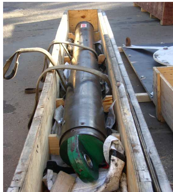
Figure 2. VTB 200 kip damper SN#009 as received at UCSD. Note displaced and rotated sleeve cover due to sheared bolts.
