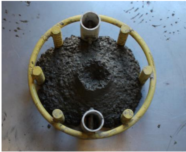
Figure 3.1 – C-Bar and L-Box Tests on Mix 4 for Pile Specimens #1 and #2
