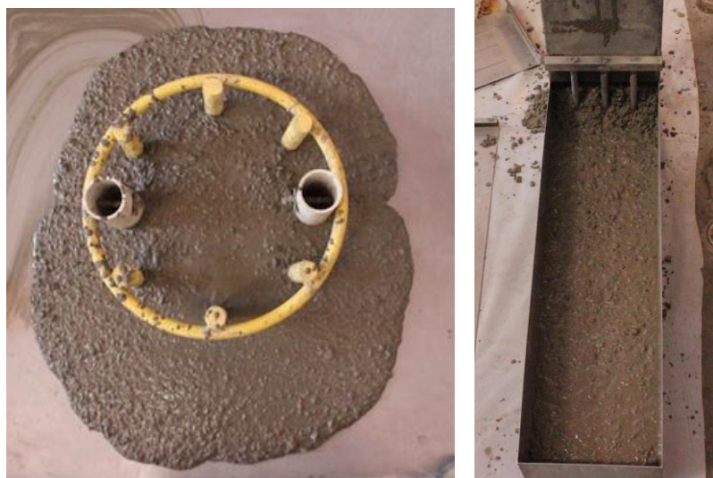
Figure 3.12 – C-Bar and L-Box tests on Caltrans Mix for Pile Specimens #7 and #8
