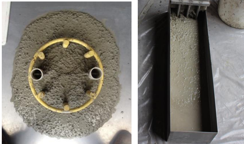
Figure 3.16 – C-Bar and L-Box tests on Mix 2 for Pile Specimens #9 and #10
