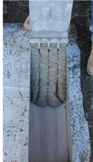
Figure 3.5 – C-Bar and L-Box tests on Mix 5 for Pile Specimens #3 and #4
