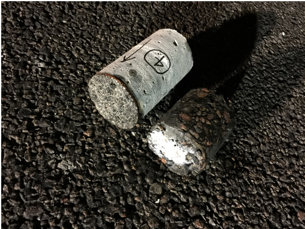
Figure 4-13. Collected concrete core
