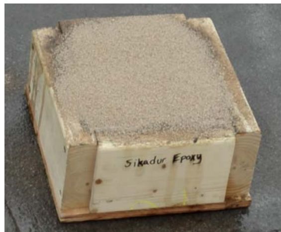
Figure 3-1. Sikadur 55SLV lab specimen
