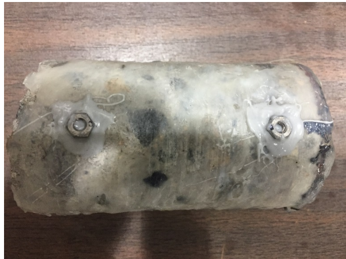
Figure 3-10. Sample prepared for freeze-thaw test
