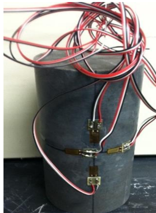
Figure 3.6. Strain gauges on specimen
