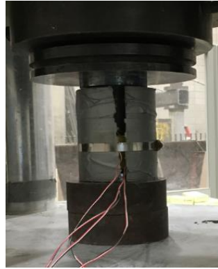
Figure 3.5. Compressive strength test setup
