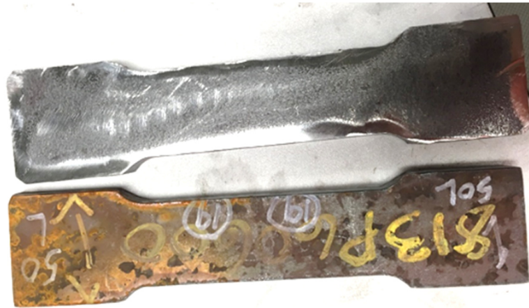
Figure 39. Corroded (bottom) and uncorroded (top) steel surfaces
