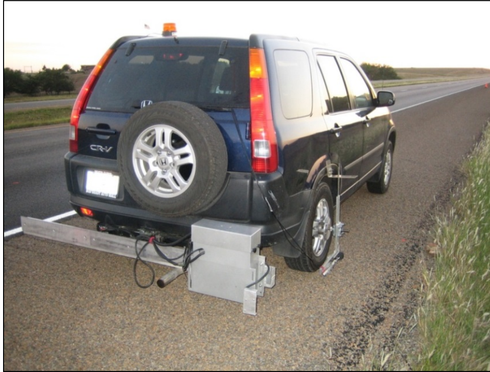
Figure 12. Photo. High-speed inertial profiler mounted behind the test vehicle.
