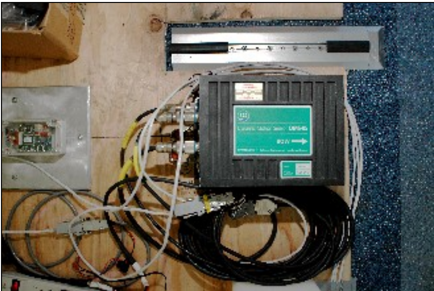
Figure 6-6. Dynamic motion sensor installed on M/V Spirit. The sensor signal was multi-plexed with signals from Real-Time Kinematic GPS, and compass
