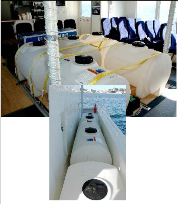
Figure 6-8. Water tanks used for ballast on board the research test vessel M/V Spirit
