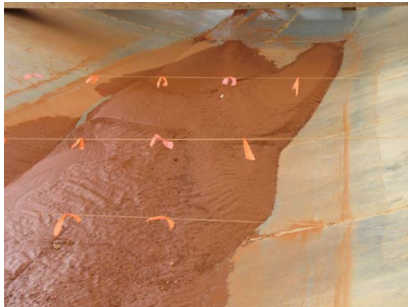
(a) Erosion Eel sediment-laden test deposition
