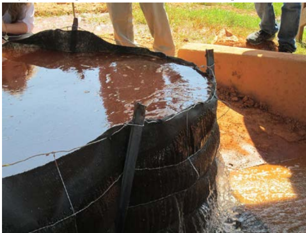
(c) strain on t-posts from full impoundment pressure
