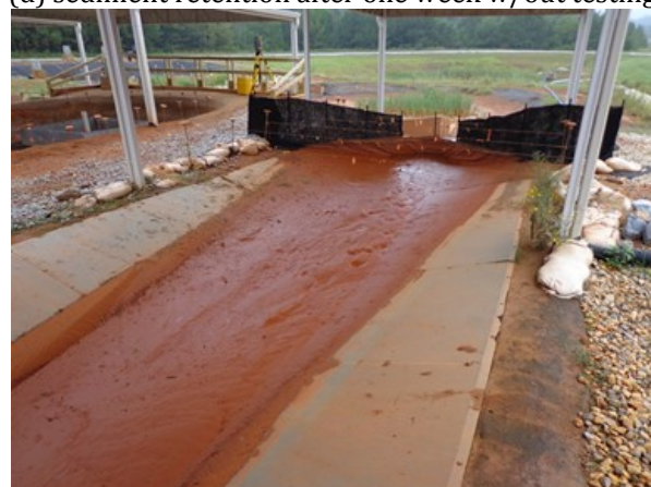
(f) sediment deposition post longevity test
