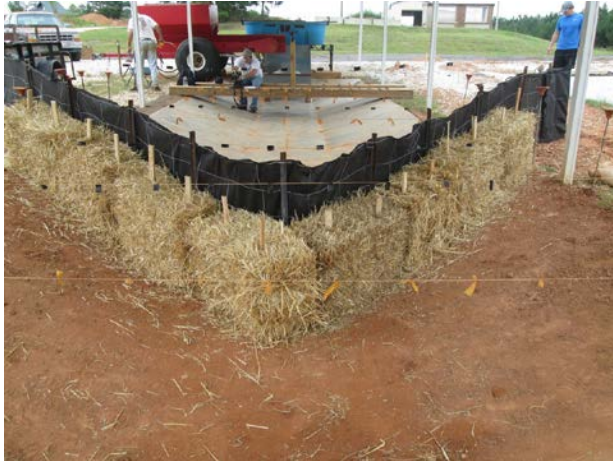
(a) hay bale dissipater pretest
