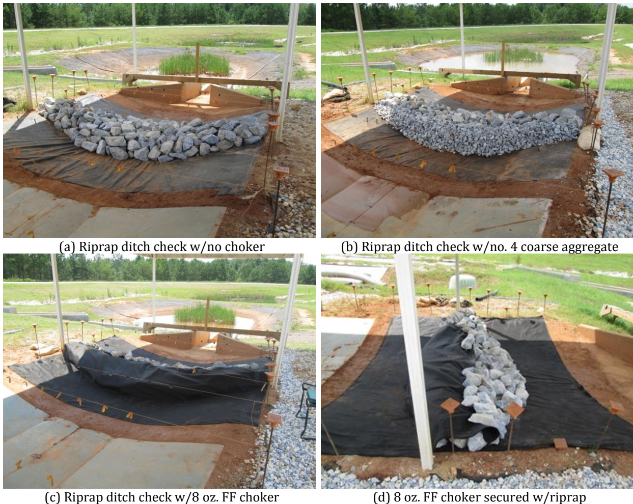
Figure 3.2: Riprap Ditch Check Installation Configurations
