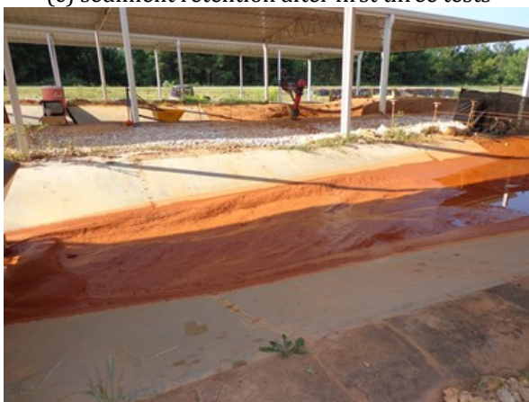
(e) large particles deposited at channel head
