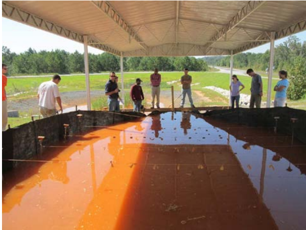
(a) full height silt fence ditch check impoundment
