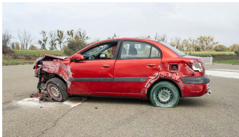
Figure 5-11 140MASH3C16-04 Kia Rio Driver Side Damage
