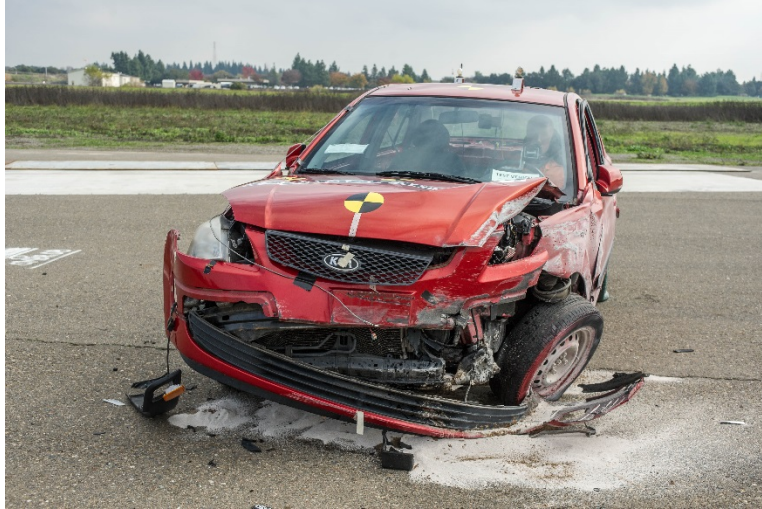
Figure 5-12 140MASH3C16-04 Kia Rio Damage (Front)
