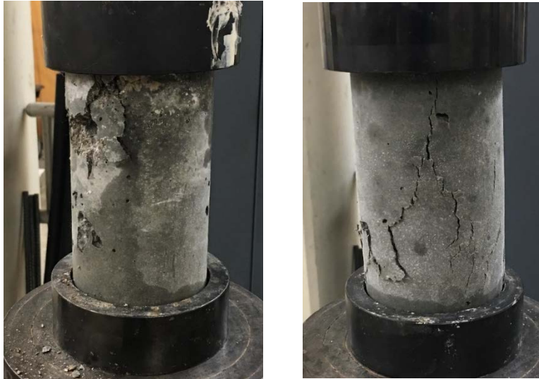
Figure 9. Concrete Specimens after Failure; Left-Control, Right-With RC2%
