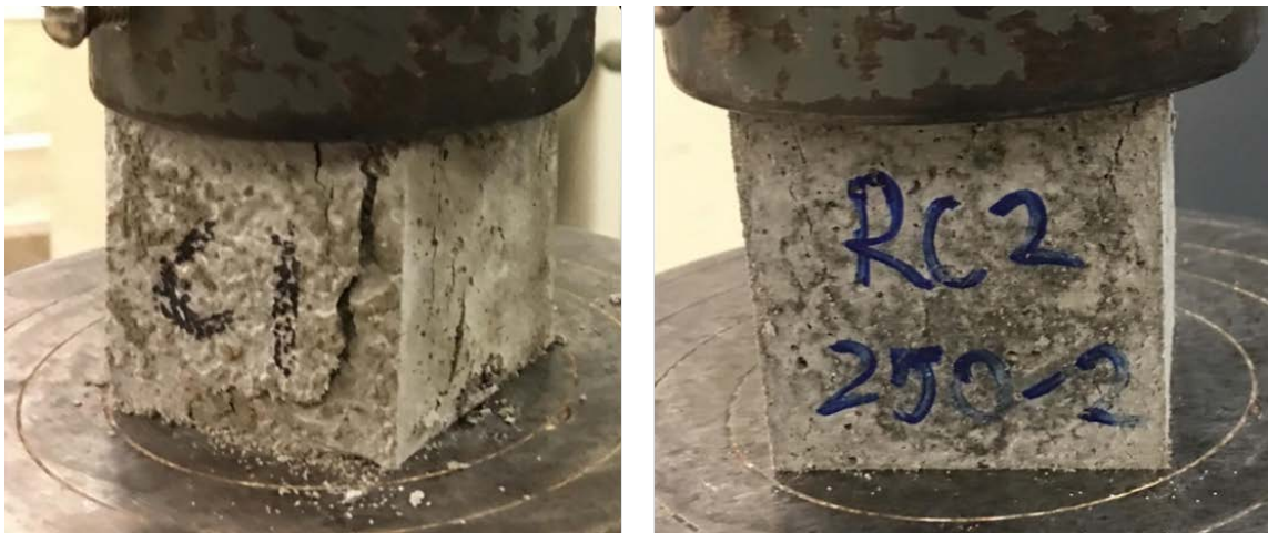
Figure 5. Mortar Specimens after Failure; Left-Control, Right-With RC2%
