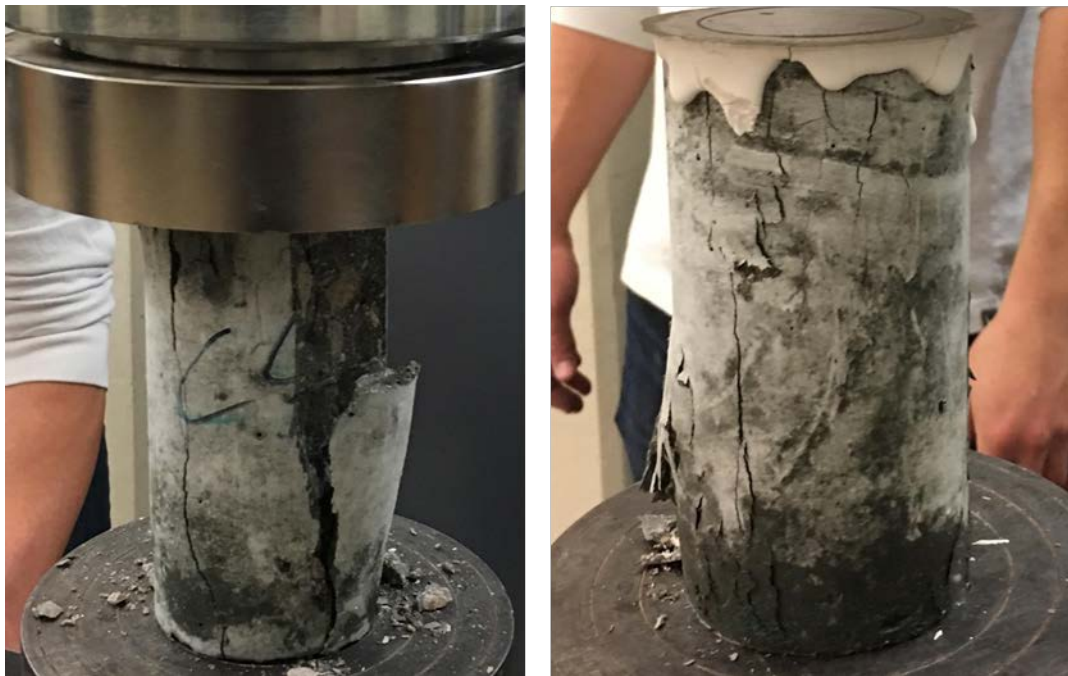
Figure 17. Concrete Specimens after Failure; Left-Control, Right-With 1% 1-inch Twisted Cotton Fibers
