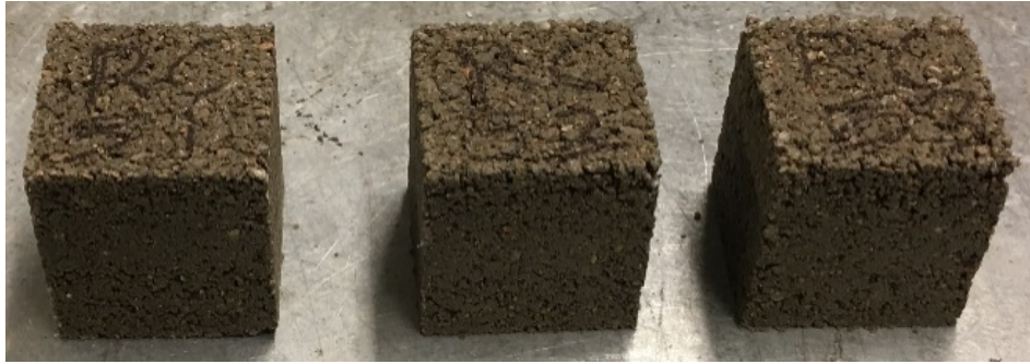
Figure 2. Cotton Mixed Mortar Specimens with No Extra Water
