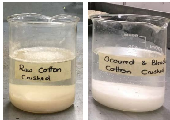
Figure 1. Water Absorbency of: Left-Crushed Row Cotton, Right-Crushed Treated Cotton
