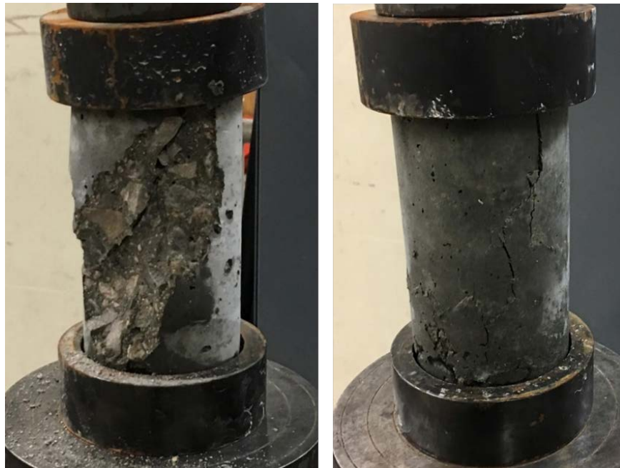
Figure 15. Concrete Specimens after Failure; Left-Control, Right-With 1% 1-inch Cotton Fibers
