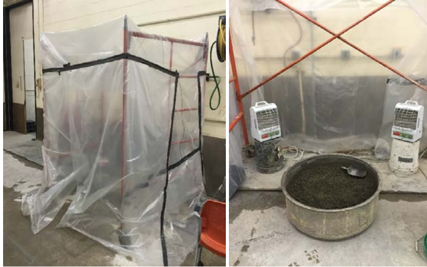
Figure M3. Thermally-controlled area for high temperature compaction delay times.
