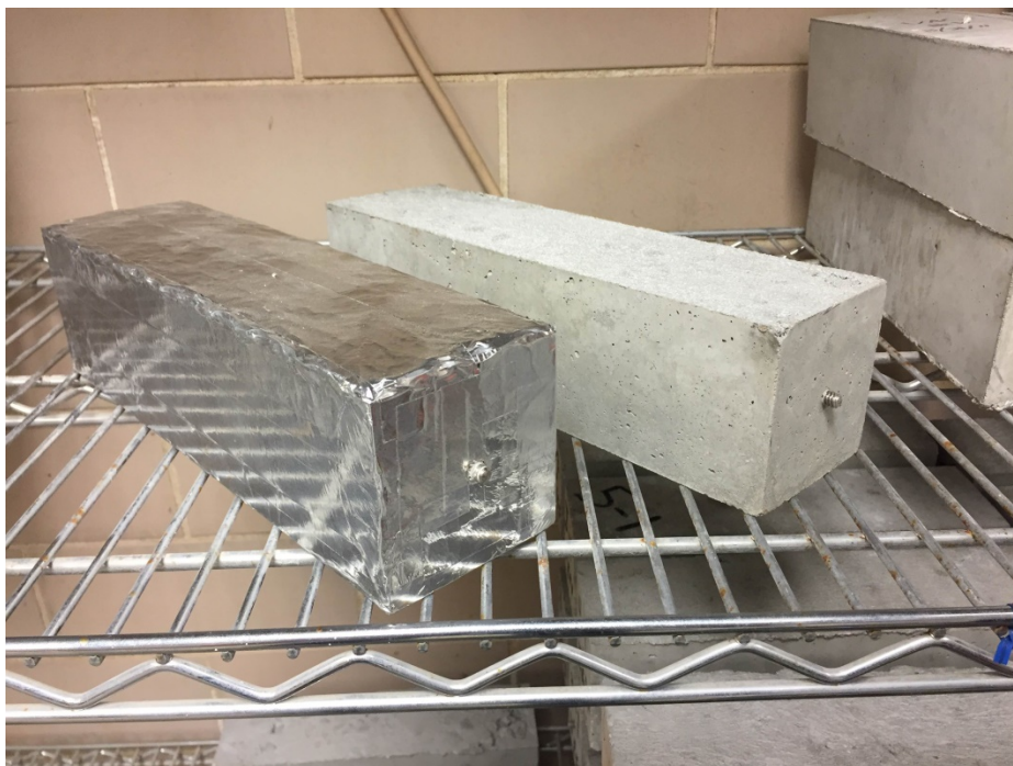
Figure K10. Sealed (left) and Drying (right) RCC Shrinkage Specimens.
