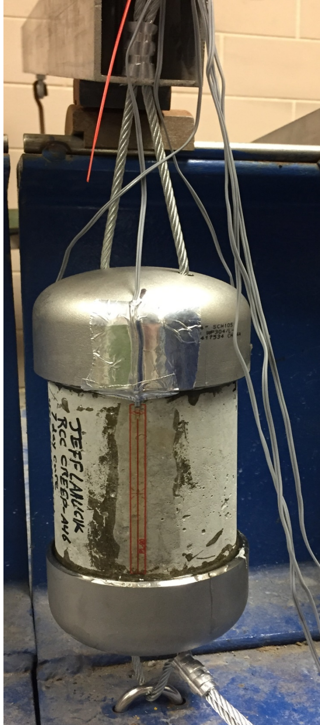
Figure K7. Tensile Creep Specimen Loaded in Cantilevered Dead Load Frame.
