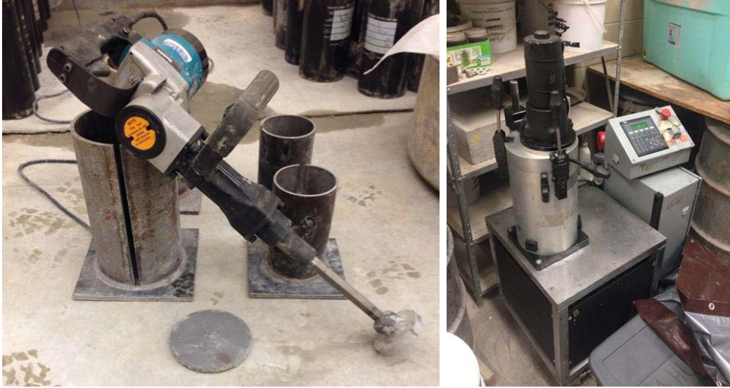
Figure M1. Vibratory Hammer (left) and Portable Gyrotory Compactor (right).
