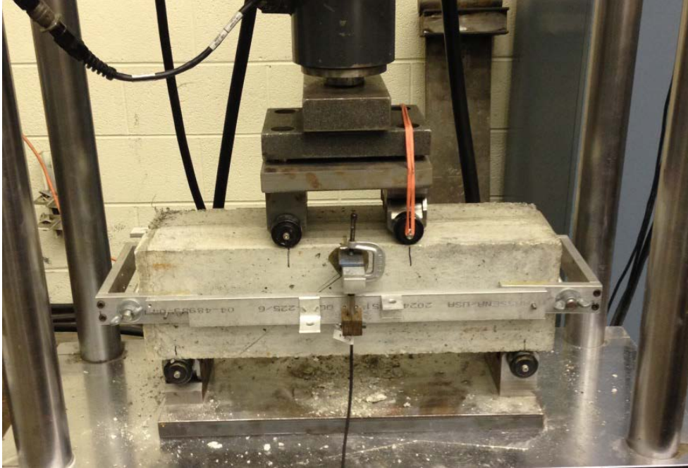
Figure I8. Flexural Performance Test Setup.
