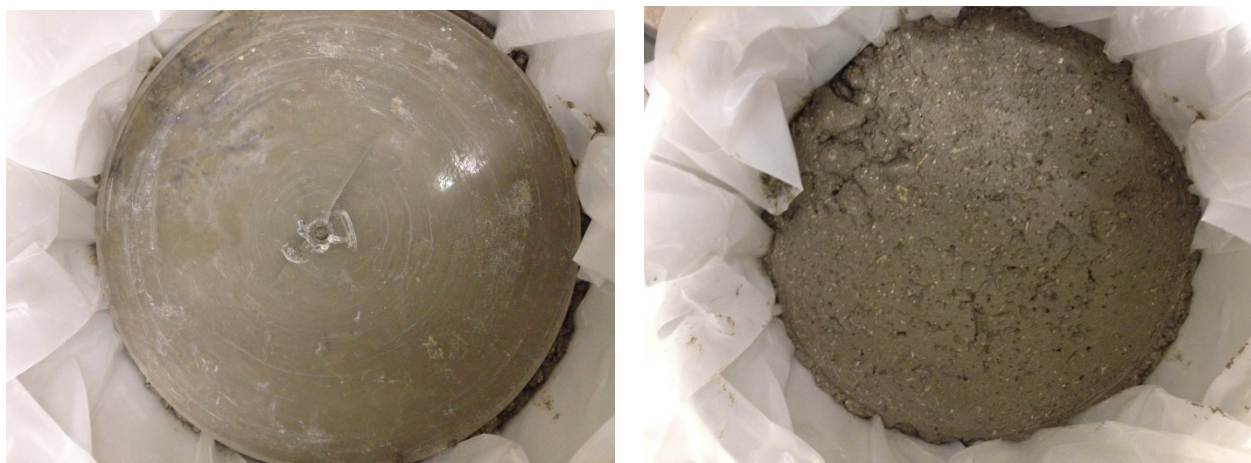
Figure 4. Compacted vebe specimen with mortar ring around plate (left) and RCC surface appearance after testing (right).
