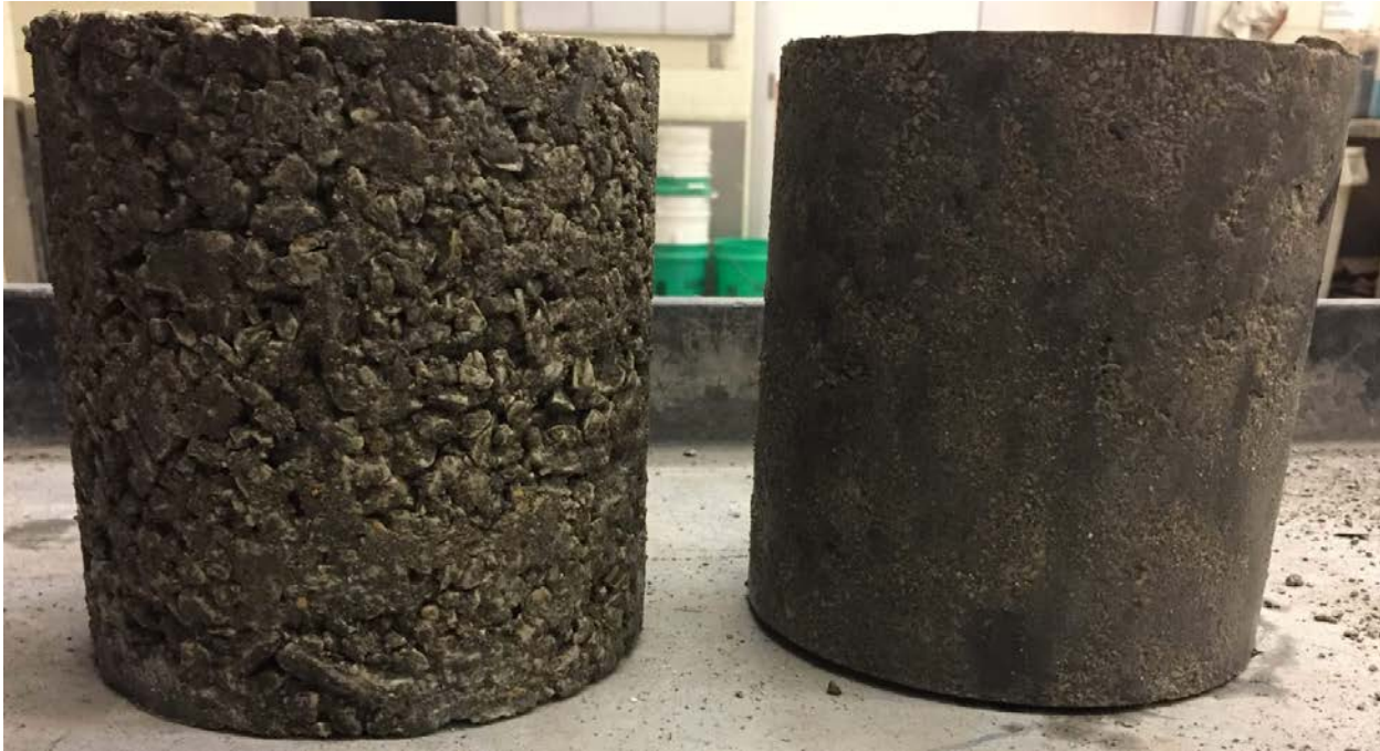
Figure L10. Specimens Compacted with Gyratory Compactor. Specimen on left (mix 9) did not meet 98% Compaction Requirement while Specimen on right did (site B mix).
