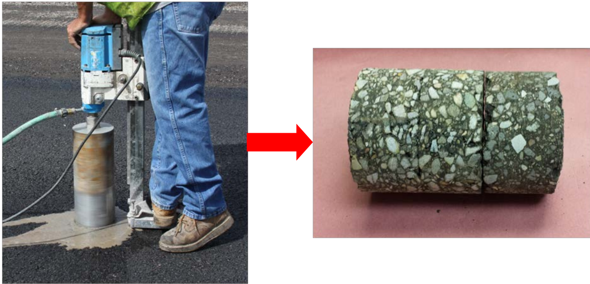
Figure 16: Extraction of field-compacted AC core
