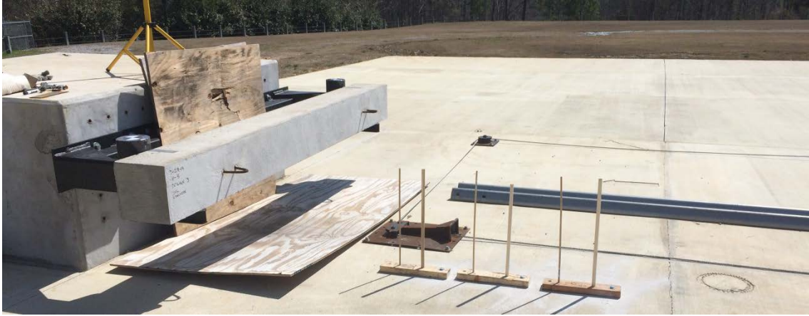
Figure 10. Beam Test Setup with Speed Dowels and Track Guidance
