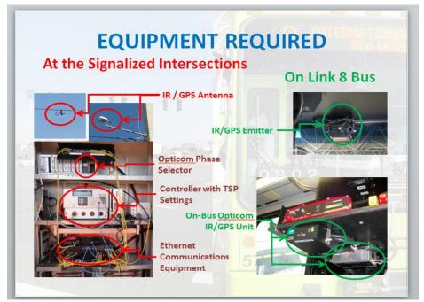
Figure 4: TSP equipment required (source: Kittleson and Associates 2013)
