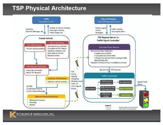
Figure 6: TSP system architecture developed by Kittleson and Associates
