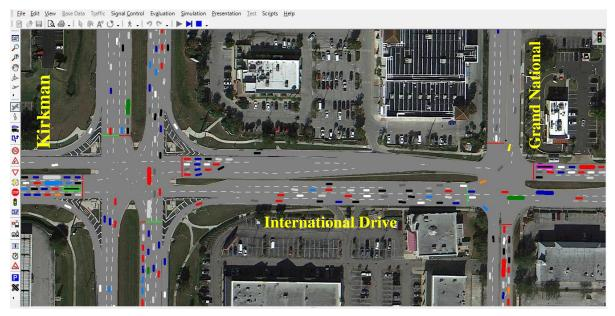
Figure 21: Kirkman and Grand National intersections on I-Drive coded in VISSIM
