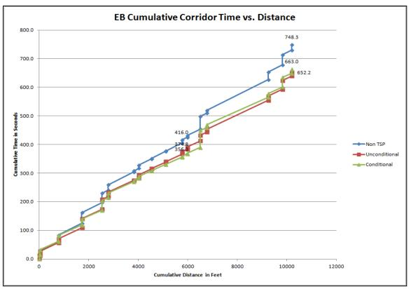
Figure 15: Eastbound bus trajectories for No TSP, Unconditional TSP, and Conditional TSP
