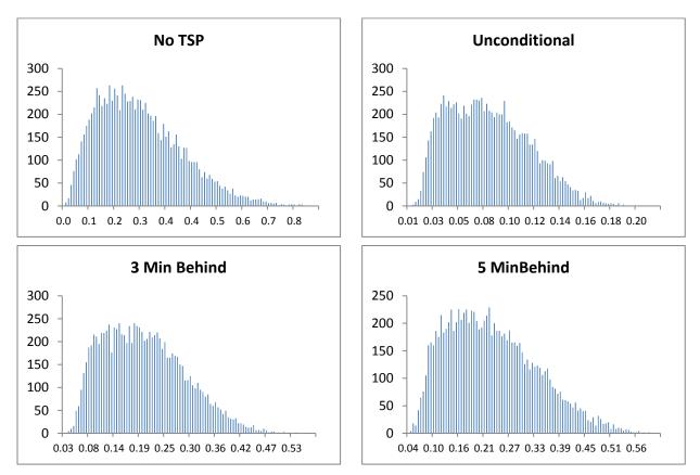
Figure 31 – Histogram of VOC emissions in idling phase for different TSP Scenarios, in grams
