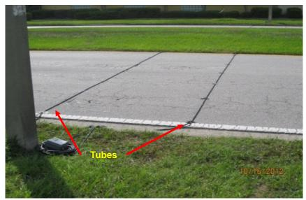
Figure 8: Pneumatic tubes used for vehicle classifications near Fun Spot Way (formerly Touchstone Drive) on northbound I-Drive
