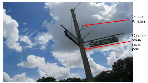
Figure 5: TSP antenna (Opticom GPS) at Del Verde Way and I-Drive
