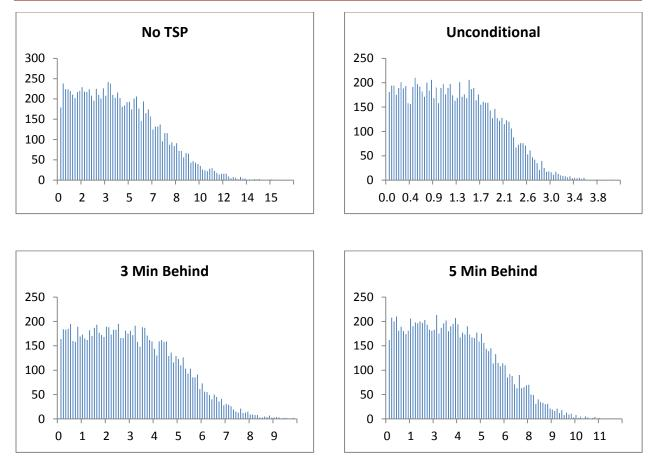
Figure 30 – Histogram of CO Emissions in idling phase for different TSP scenarios, in grams
