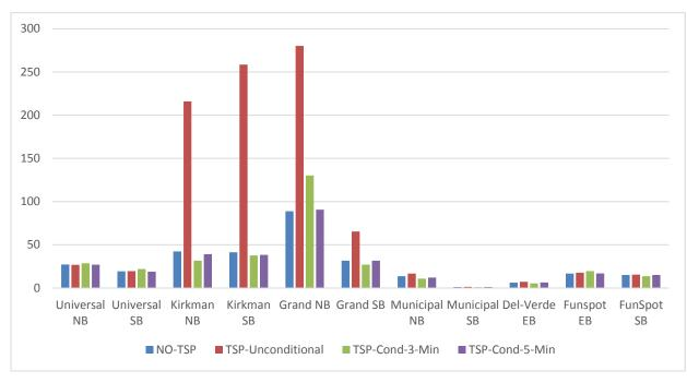
Figure 27: Crossing streets average delay per vehicle in seconds
