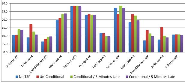
Figure 26: Average speeds (ft/sec) at signalized intersections
