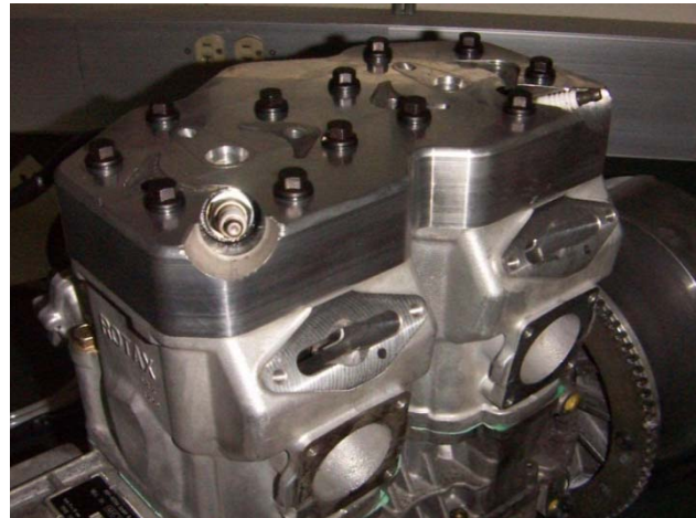
Figure 3: Completed UICSC DI head installed on the Rotax 600 H.O. engine.
