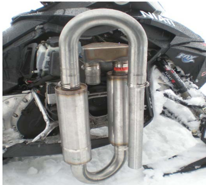
Figure 17: Two Hushpower mufflers in series mounted on the UICSC snowmobile for sound testing.
