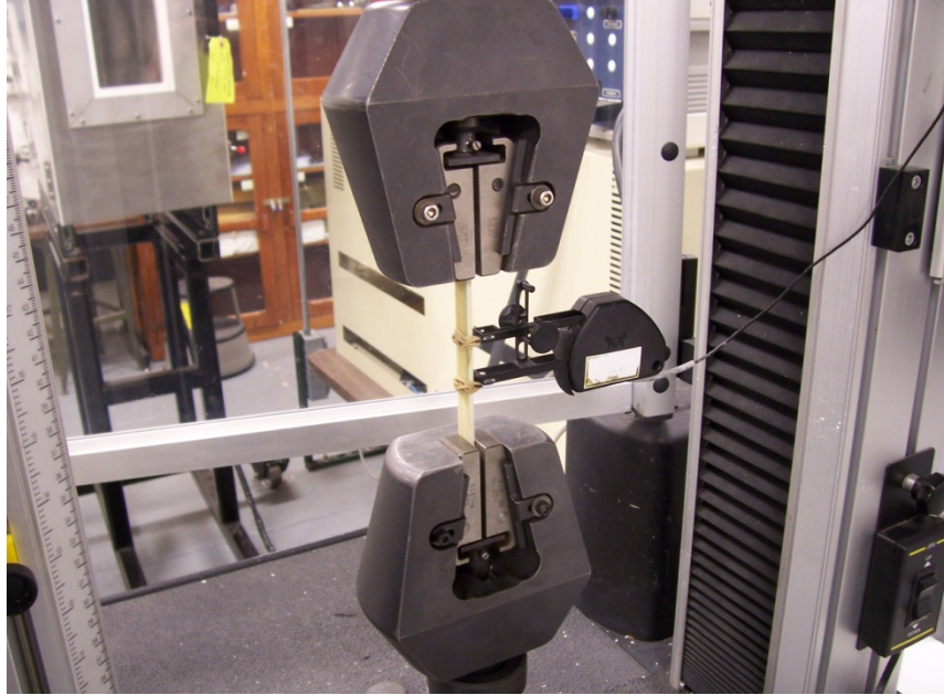
Figure 2. Tensile test setup at Missouri S&T
