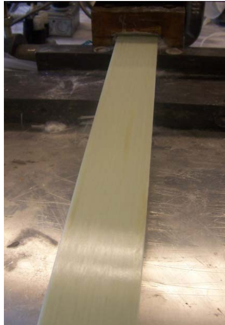
Figure 4. Pultruded aliphatic PU composite manufactured at Missouri S&T
