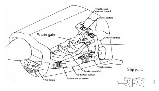
Figure D-5. Six-Cylinder, Horizontally Opposed Turbocharged Engine [D-1]
