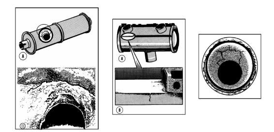
Figure C-4. Typical Muffler Failures [C-7] (Exhaust Outlet Fatigue (Left), Wall Fatigue (Middle), and End Plate Fatigue at Inlet (Right))
