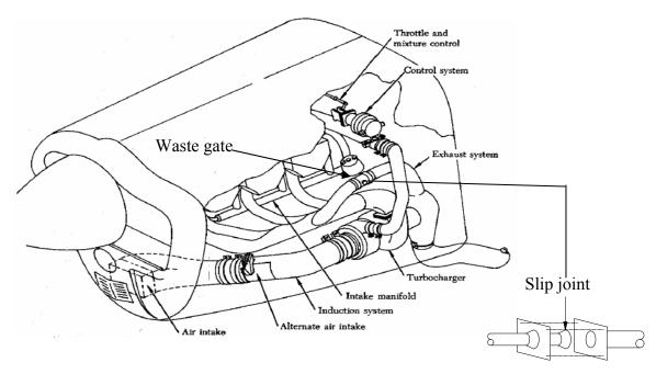
Figure C-5. Six-Cylinder, Horizontally Opposed Turbocharged Engine [C-1]
