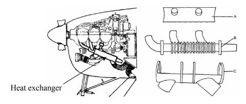
Figure 1. Six-Cylinder, Horizontally Opposed Reciprocating Engine [5] (Heat Exchanger Upper Sheet Jacket (A), Collector Tube (B), and Lower Sheet Jacket (C))
