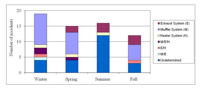
Figure A-5. Seasonal Distribution of CO-Related Accidents and Their Source of CO Leakage
