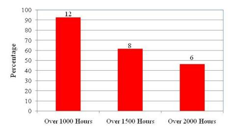
Figure A-10. Percentage of GA Aircraft CO-Related Accidents/Incidents as a Function of Hours of Muffler Use
