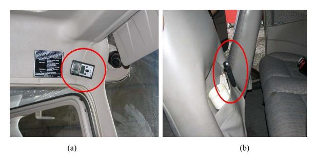
Figure B-3. Carbon Monoxide Detectors Located (a) Near the Pilot-Side Visor and (b) the Back-Seat Area With Suspender Clips
