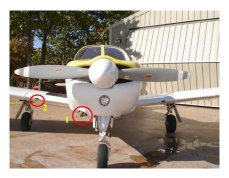
Figure C-11. Piper PA-28 Locations for the Exhaust Tailpipe (1) and Fresh Air Inlet (2) [C-19]
