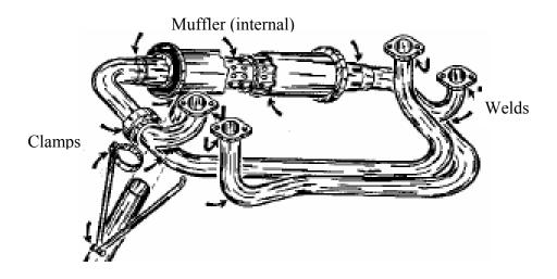
Figure C-2. Typical Exhaust System Inspection Areas [C-1]
