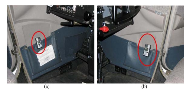
Figure B-2. Carbon Monoxide Detectors Attached to the Left-Door Pocket (a) and Right-Door Pocket (b) With Suspender Clips
