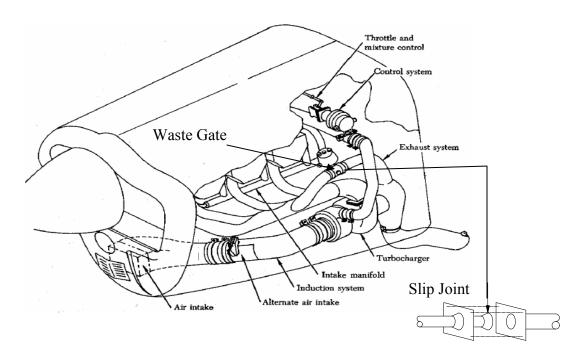
Figure 5. Six-Cylinder, Horizontally Opposed Turbocharged Engine [5]
