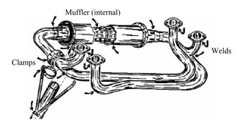
Figure 2. Typical Exhaust System Inspection Areas [5]
