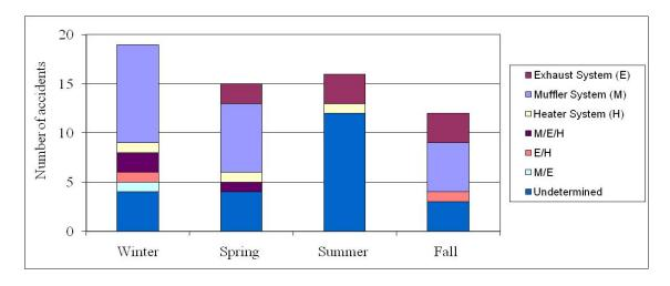
Figure C-9. Seasonal Distribution of CO-Related Accident/Incidents and Their Source of CO Leakage
