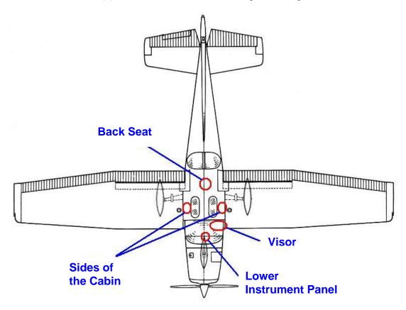
Figure B-4. Top View of CO Detector Locations in the High-Wing Aircraft Model
