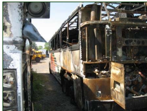
Figure 6. Left rear view of the fire damage to the motorcoach.
