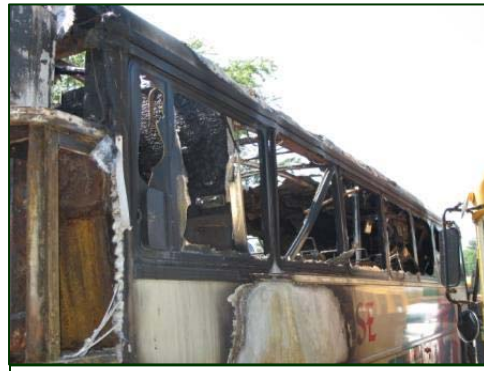
Figure 15. Right side glazing damage.
