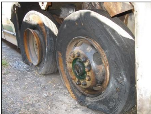
Figure 5. Fire damage to the left drive and tag axle tires.
