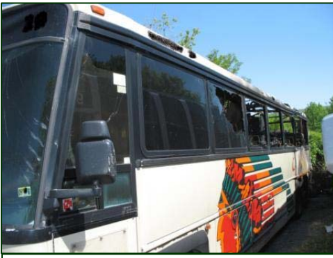
Figure 14. Left side glazing damage.
