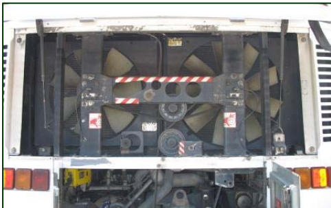
Figure 9. Aluminum AC condenser (left) and radiator (right) of the exemplar motorcoach.
