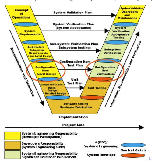
It is important to keep in mind that CM does not exist in isolation. It is an important and integral component of the systems engineering process. This means that CM begins when the system concept is formulated and then "follows through" for the entire system life-cycle.
