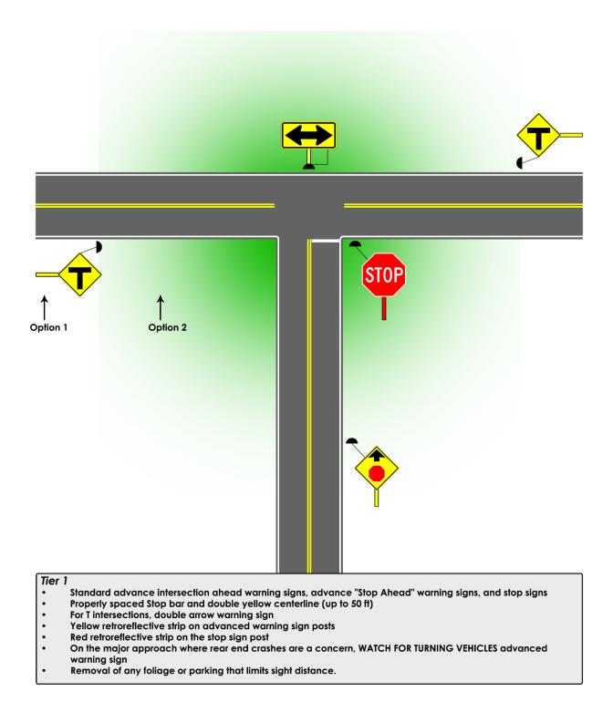
Figure 7. Tier 1 Countermeasures for 3-Leg Intersections. (For 4-leg intersections, remove the double arrow and duplicate the stop sign approach on the opposite side.)
