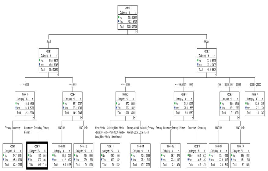
Figure 4. Classification Tree for FOOR Collisions at 3-Leg Unsignalized Intersections. FOOR = fixed object off road.
