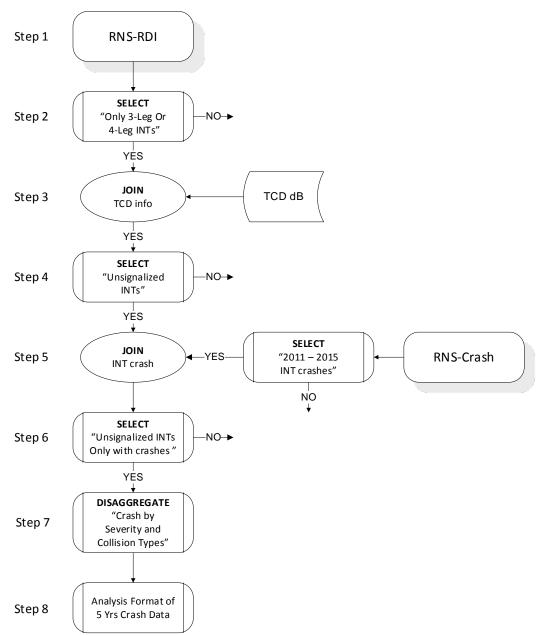
Figure 1. Procedure for Identifying Focus Collision Types at Unsignalized Intersections
