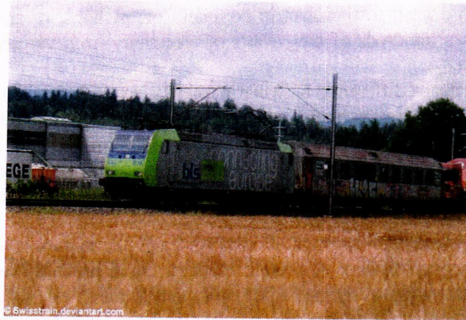
FIGURE 24 Bombardier TRAXX 140 AC – Re 485.
