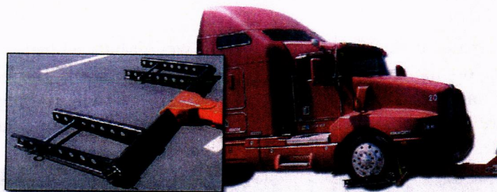
FIGURE 20 An example of a board to tie down vehicles (14).
