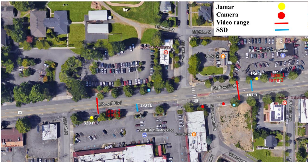
Figure 5.8: Location of data collection equipment at SE Powell Blvd. and SE 36th Ave.
