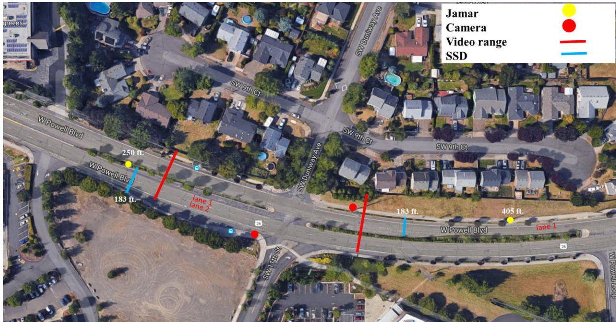
Figure 5.16: Location of data collection equipment at W. Powell Blvd. and SW Duniway Ave.
