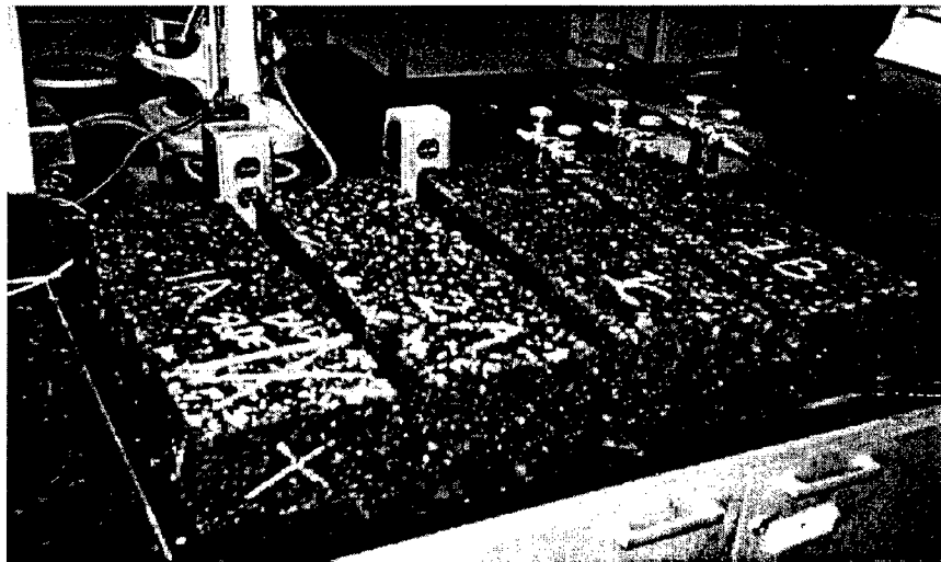
Figure 4.3 Beams compacted by CDOT Linear Kneading Compactor
