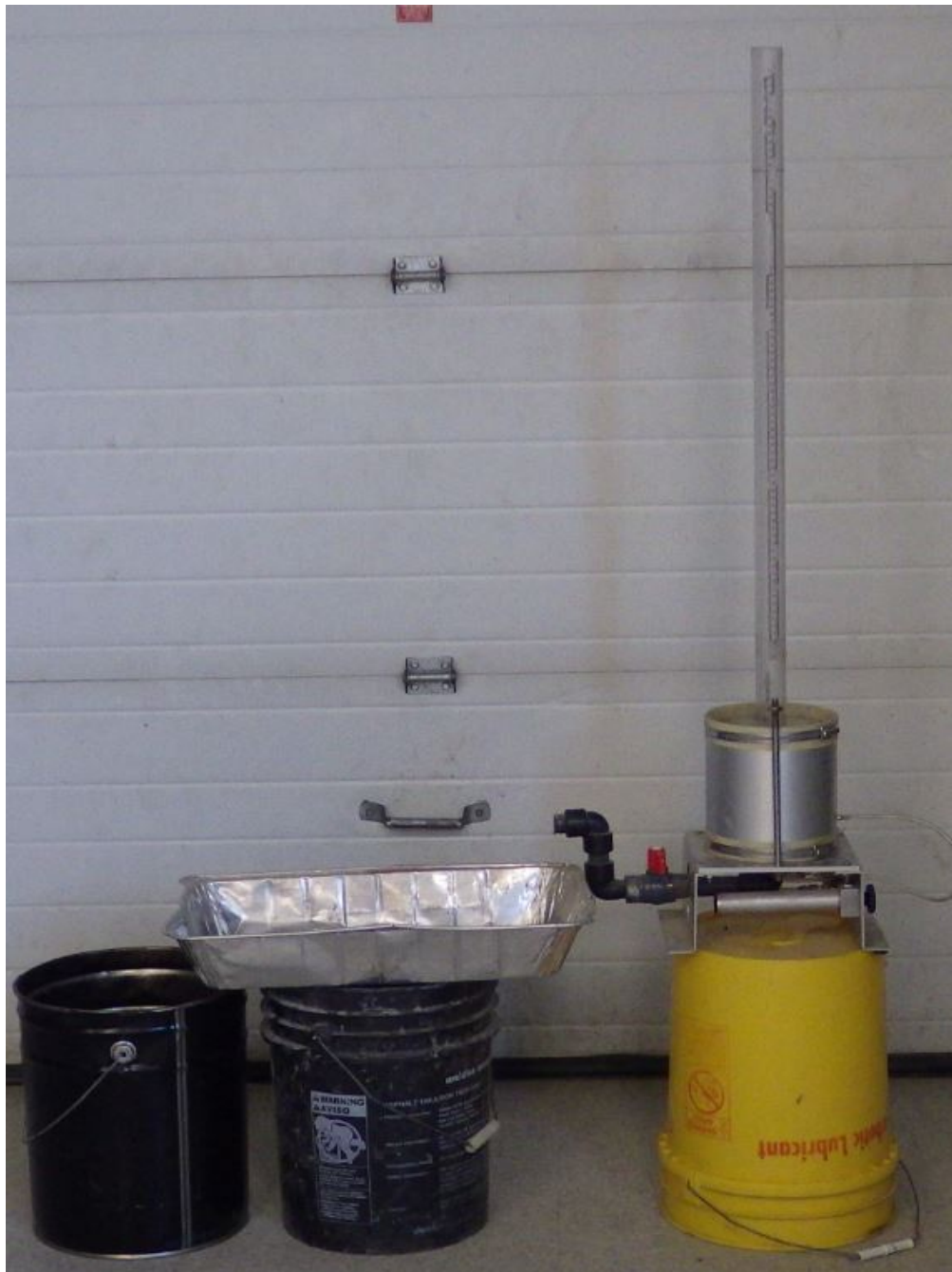
Figure 3. Laboratory Permeability Assembly
