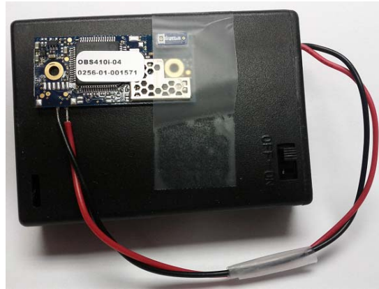
Figure 3-4 A Bluetooth Beacon Prototype Powered by 3 AA Batteries
