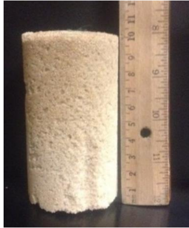
Figure 6. Cemented sand after MICP treatment
