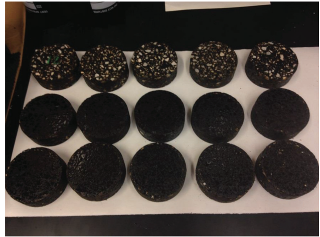
Figure 3.3 Asphalt mixture specimens after first conditioning treatment.
