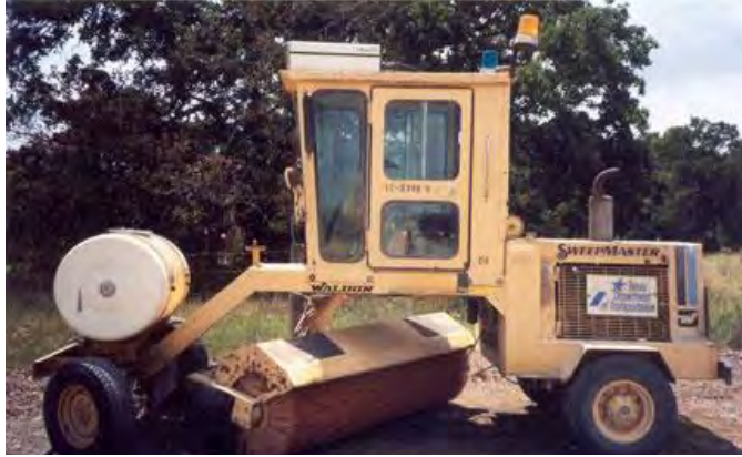
Figure 3 - Road Sweepers for Cleaning Pavement Surface [6]
