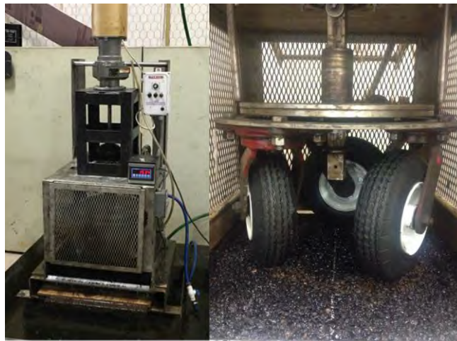
Figure 1 - Polish Test Device (PTD) (left: overall view of the device; right: closer view of the wheels)
