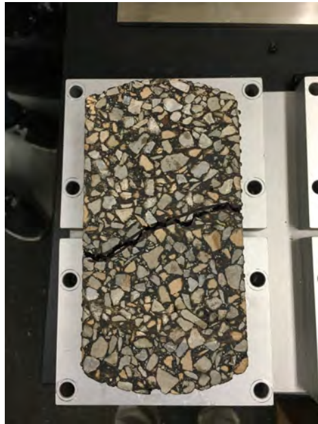
Figure 5.4. Cracked Overlay Test Specimen
