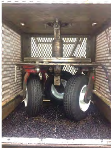
Figure 4.2. Thin asphalt layer being tested under the three wheel polishing device
