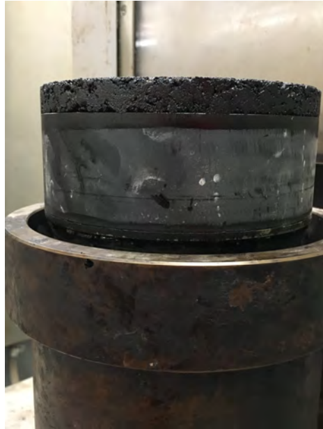
Figure 5.2. Thin Asphalt Layer Applied to a Polymer Base for Modified Hamburg Wheel Tracking Test
