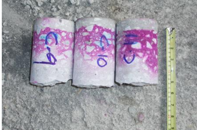
Figure 4-1 Phenolphthalein Indicator Solution on Concrete Core (Parrott, 1987)
